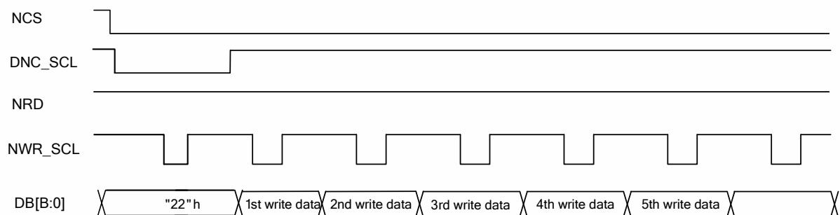
**Read the graphic RAM**
