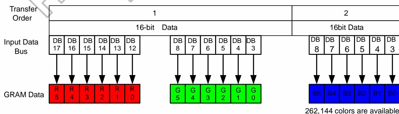
**Figure 5.14 Input data bus and GRAM data mapping in 16-bit bus system interface with 18(12+6) bit-data input (R17H=06h and “IM3, IM2, IM1, IM0”=”0010”)**
