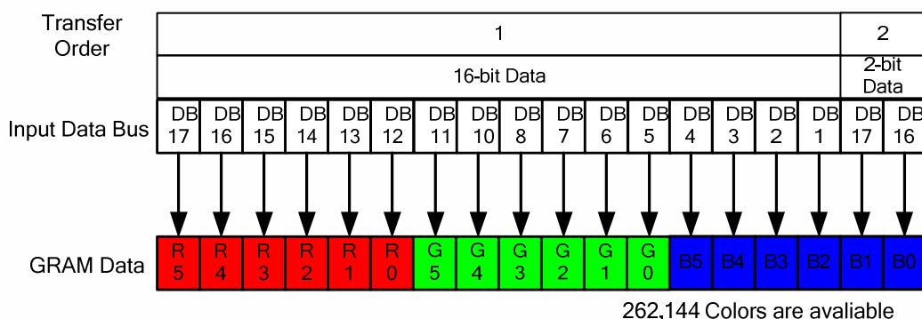
**Figure 5.15 Input data bus and GRAM data mapping in 16-bit bus system interface with 18(16+2) bit-data input (R17H=07h and “IM3, IM2, IM1, IM0”=”0010”)**
