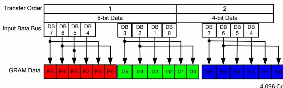
Figure 5.23 Input data bus and GRAM data mapping in 8-bit bus system interface with 12 bit-data input (R17H=03h and “IM3, IM2, IM1, IM0”=“0001”)
