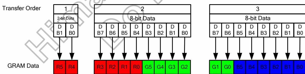
Figure 5.26 Input data bus and GRAM data mapping in 8-bit bus system interface with 18(2+8+8) bit-data input (R17H=07h and “IM3, IM2, IM1, IM0”=“0001”)
