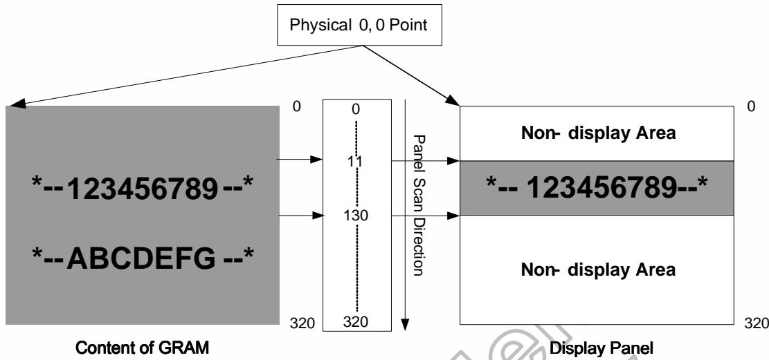
**Figure 6.5 Partial display when  $ML = '0'$**
