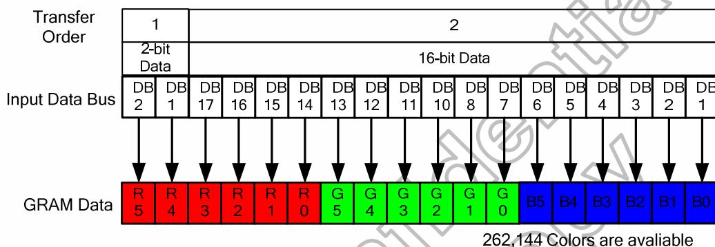
**Figure 5.16 Input data bus and GRAM data mapping in 16-bit bus system interface with 18(2+16) bit-data input (R17H=04h and “IM3, IM2, IM1, IM0”=”0010”)**
