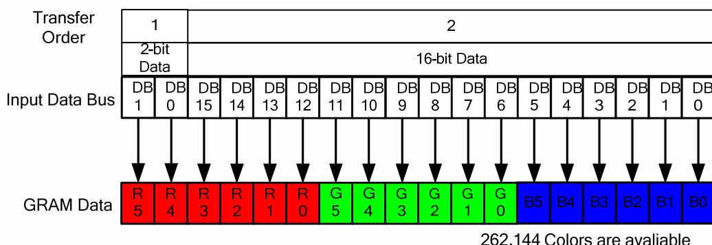
**Figure 5.11 Input data bus and GRAM data mapping in 16-bit bus system interface with 18(2+16) bit-data input (R17H=04h and “IM3, IM2, IM1, IM0”=”0000”)**
