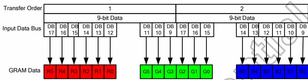
**Figure 5.20 Input data bus and GRAM data mapping in 9-bit bus system interface with 18 bit-data input
