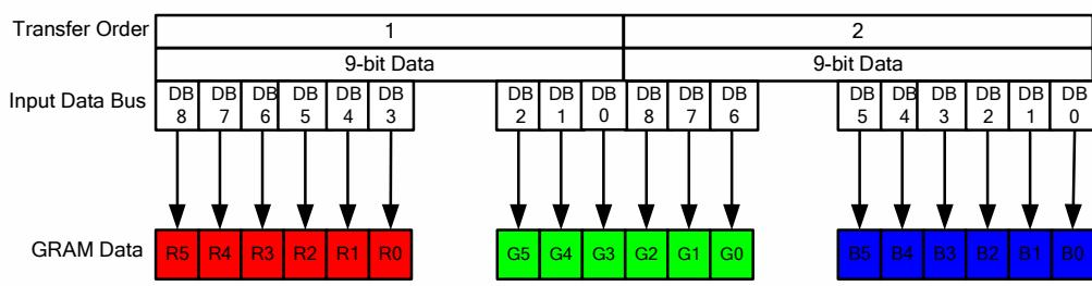
**Figure 5.19 Input data bus and GRAM data mapping in 9-bit bus system interface with 18 bit-data input
