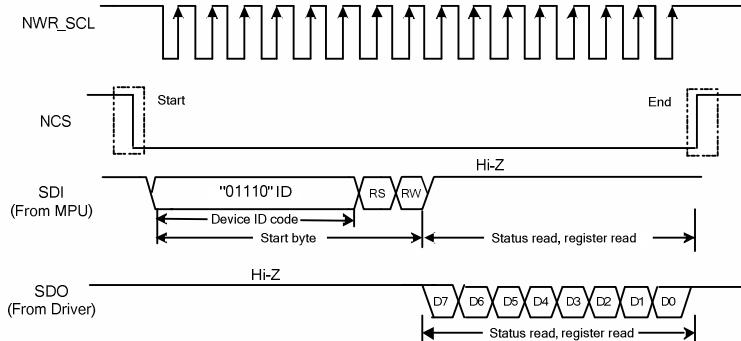
Figure 5.31 Index register read/write timing in 3-wire serial bus system interface
