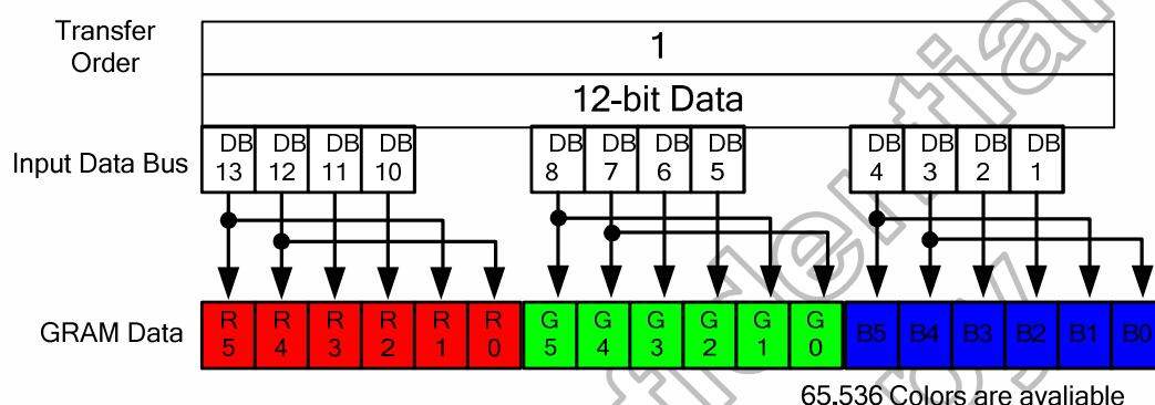
**Figure 5.12 Input data bus and GRAM data mapping in 16-bit bus system interface with 12 bit-data input (R17H=03h and “IM3, IM2, IM1, IM0”=”0010”)**
