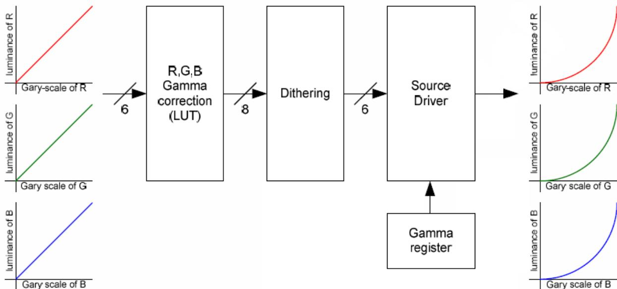
**Figure 7.7 Block diagram of digital gamma correction**
