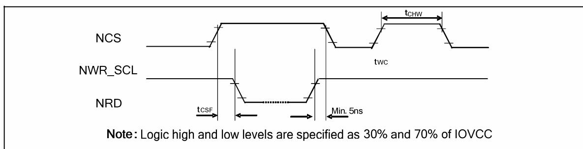
**Figure 11.2 Chip select timing**
