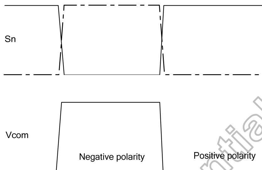
**Figure 7.5 Relationship between source output and Vcom**
