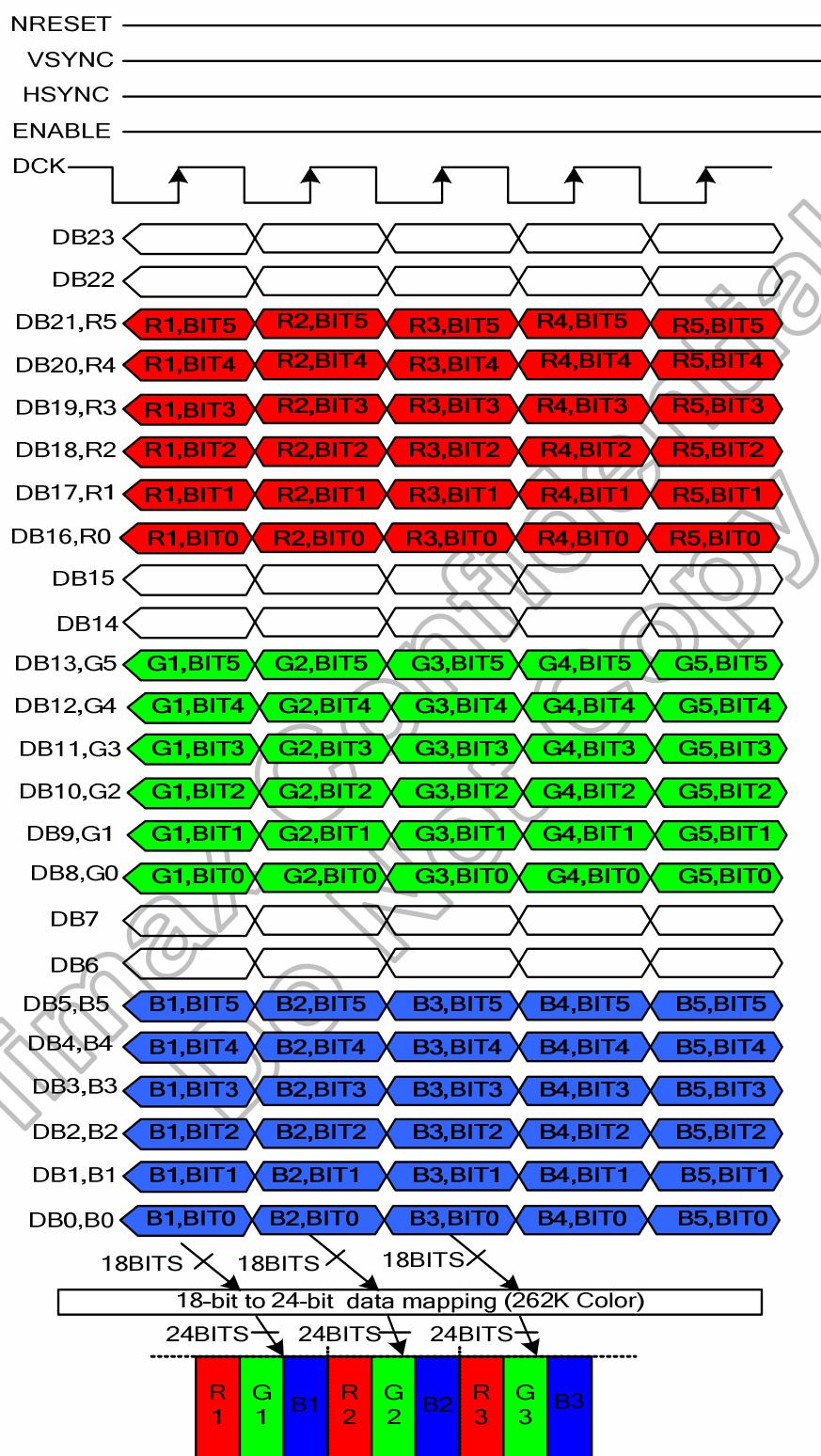
**Note:** The Data order is shown as follows, MSB = DB23, LSB = DB0 and Picture Data is MSB = Bit5, LSB = Bit0 for Red, Green and Blue data. DB23, DB22, DB15, DB14, DB7 and DB6 are opened.
