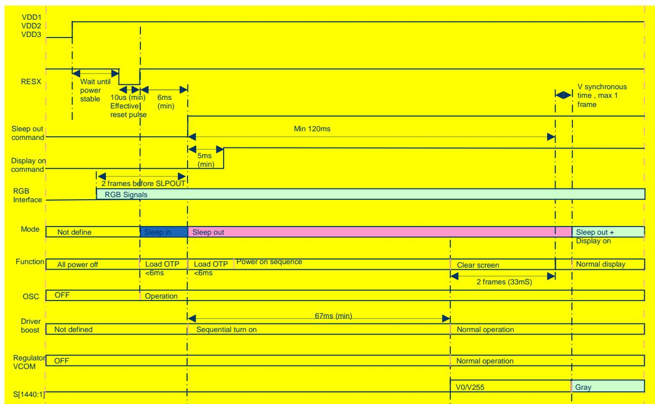
Figure 8.11 Power On Timing
