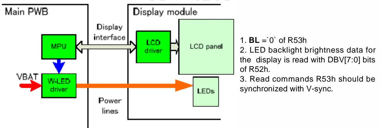
**Figure 5.15 Module architecture**
