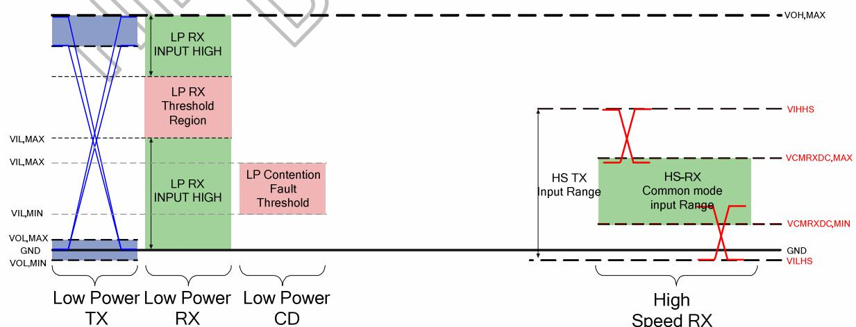
**Figure 8.6 Shows both the HS and LP signal levels**
