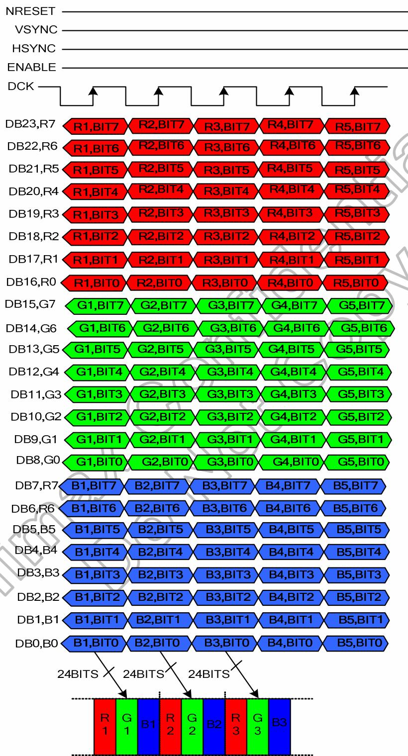
**Note:** The Data order is shown as follows, MSB = DB23, LSB = DB0 and Picture Data is MSB = Bit7, LSB = Bit0 for Red, Green and Blue data.
