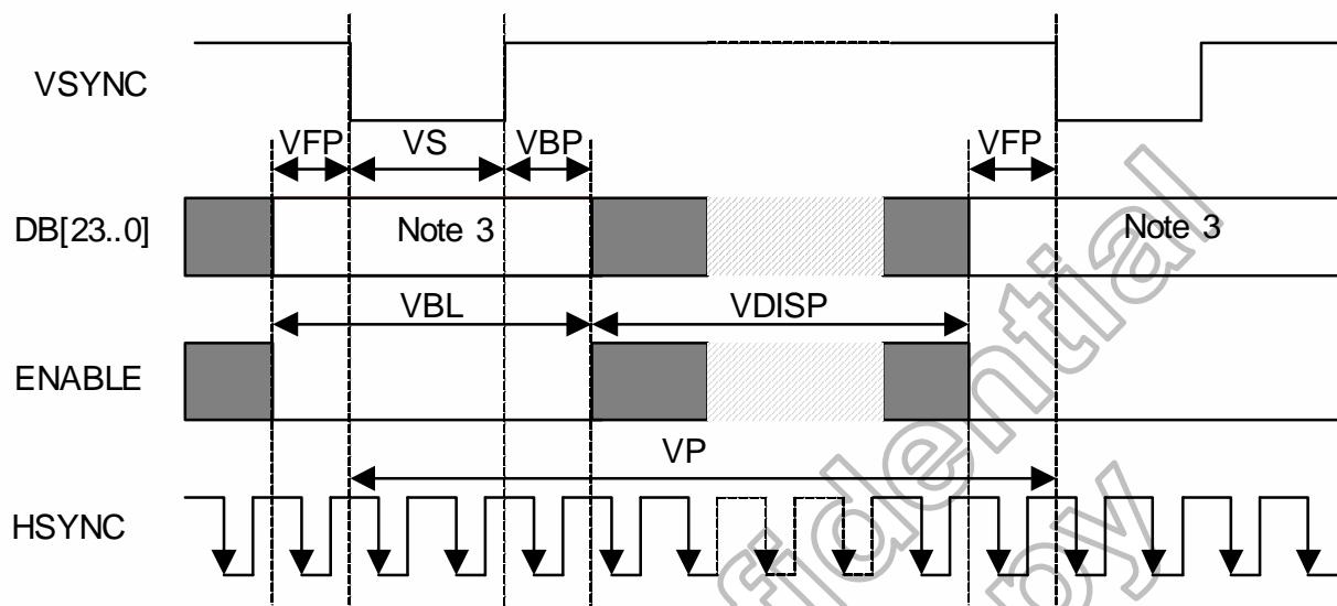
**Figure 8.2 Vertical Timings for RGB I/F**
