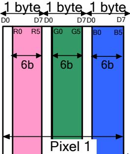
A detailed diagram showing the internal structure of a pixel. It consists of three vertical columns representing Red (R), Green (G), and Blue (B) components. Each component is 6 bits wide, labeled '6b'. The total width of the pixel is 18 bits. The bytes are labeled D0, D1, D2, D3, D4, D5, D6, and D7. The R component starts at D0 and ends at D5. The G component starts at D6 and ends at D11. The B component starts at D12 and ends at D17. The diagram is labeled 'Pixel 1'.
