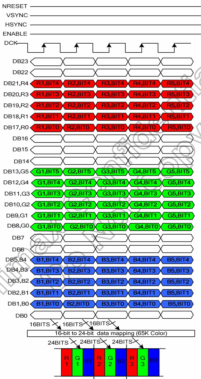
**Note:** The Data order is shown as follows, MSB = DB23, LSB = DB0 and Picture Data is MSB = Bit5, LSB = Bit0 for Green data and MSB = Bit4, LSB = Bit0 for Red and Blue data. DB23, DB22, DB16, DB15, DB14, DB7, DB6 and DB0 are opened.
