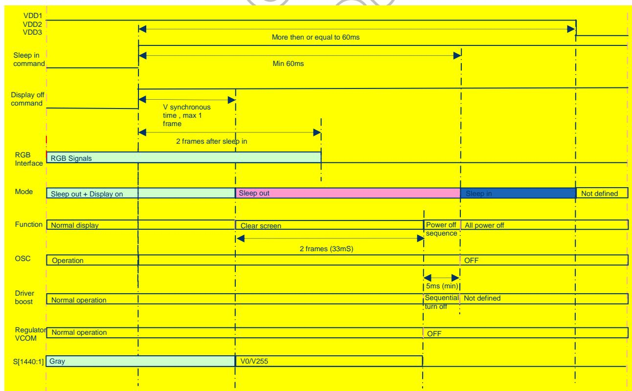
Figure 8.12 Power Off Timing
