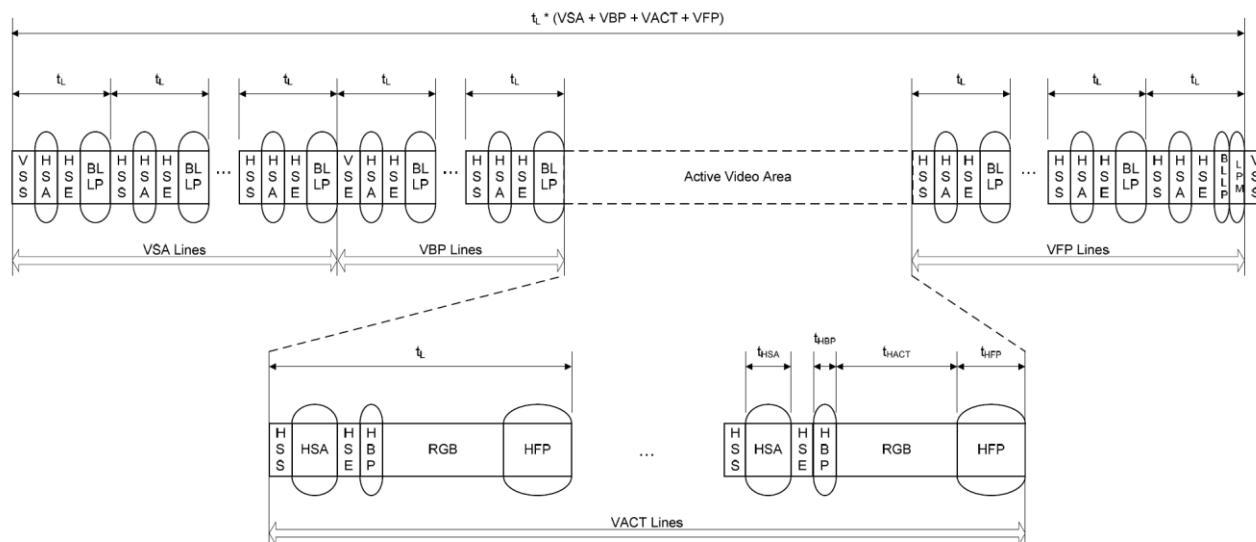
Normally, periods shown as HSA (Horizontal Sync Active), HBP (Horizontal Back Porch) and HFP (Horizontal Front Porch) are filled by Blanking Packets, with lengths (including packet overhead) calculated to match the period specified by the peripheral's data sheet. Alternatively, if there is sufficient time to transition from HS to LP mode and back again, a timed interval in LP mode may substitute for a Blanking Packet, thus saving power.
