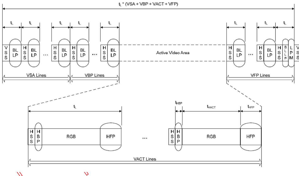
As with the previous Non-Burst Mode, if there is sufficient time to transition from HS to LP mode and back again, a timed interval in LP mode may substitute for a Blanking Packet, thus saving power.
