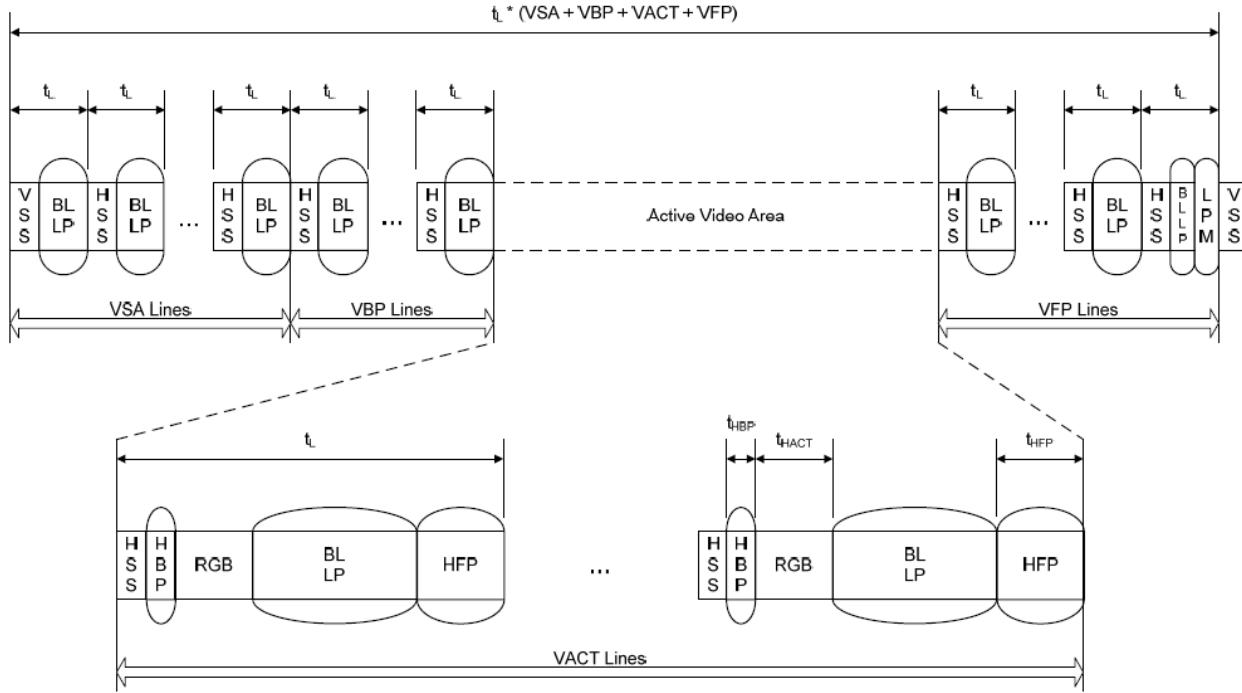
Similar to the Non-Burst Mode scenario, if there is sufficient time to transition from HS to LP mode and back again, a timed interval in LP mode may substitute for a Blanking Packet, thus saving power.
