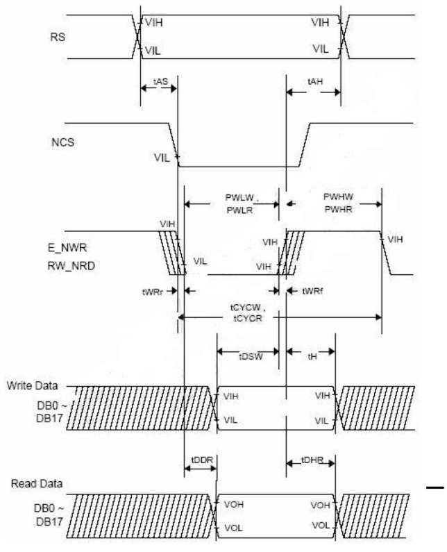
Figure 5.1:8080 System Bus Timing
