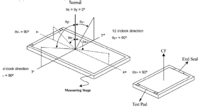
\*\*\* The above "Viewing Angle" is the measuring position with Largest Contrast Ratio; not for good image quality.
