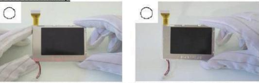
As above picture, please handle with anti-static gloves around LCM edges.
