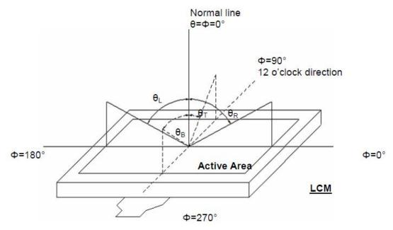
Note 2: Definition of optical measurement system.
