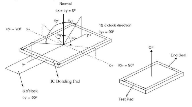
\*\*\* The above "Viewing Angle" is the measuring position with Largest Contrast Ratio; not for good image quality. View Direction for good image quality is 6 O'clock. Module maker can increase the "Viewing Angle" by applying Wide View Film.
