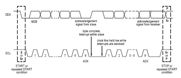
Figure 1-1 I2C Serial Data Transfer Format
