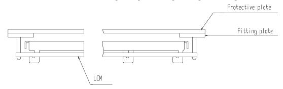
4.1.2 When assembling the LCM into other equipment, the spacer to the bit between the LCM and the fitting plate should have enough height to avoid causing stress to the module surface, refer to the individual specifications for measurements. The measurement tolerance should be  $\pm 0.1$  mm.
