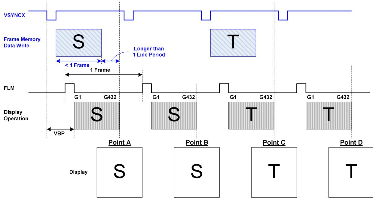
Figure 35 Operation for Leading Mode of VSYNC Interface
