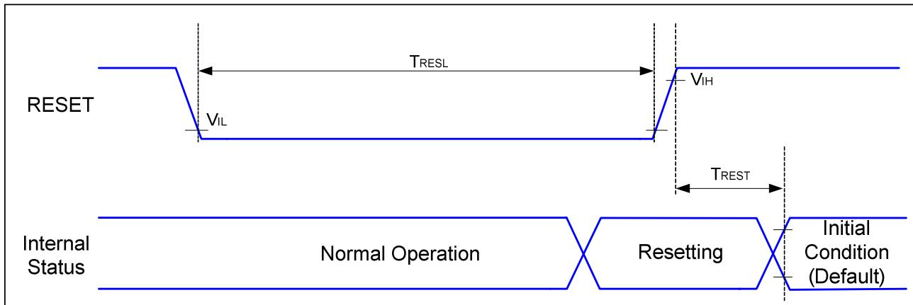
Figure 41 Reset Timing
