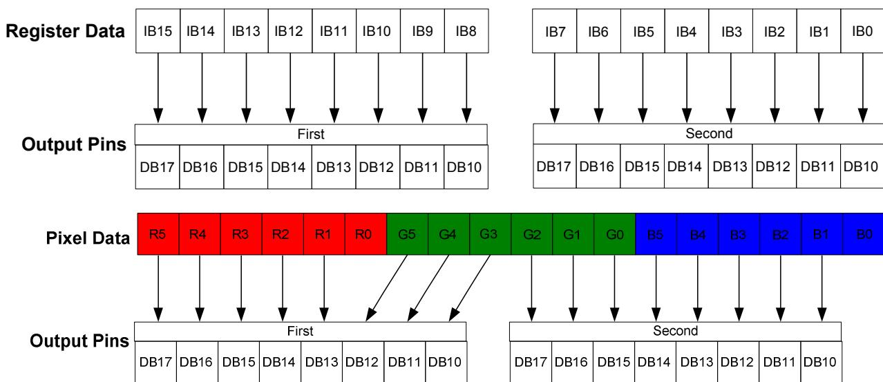
Figure 21 8-bit 8080-Series Interface Data Format (Register/Pixel Data Read)
