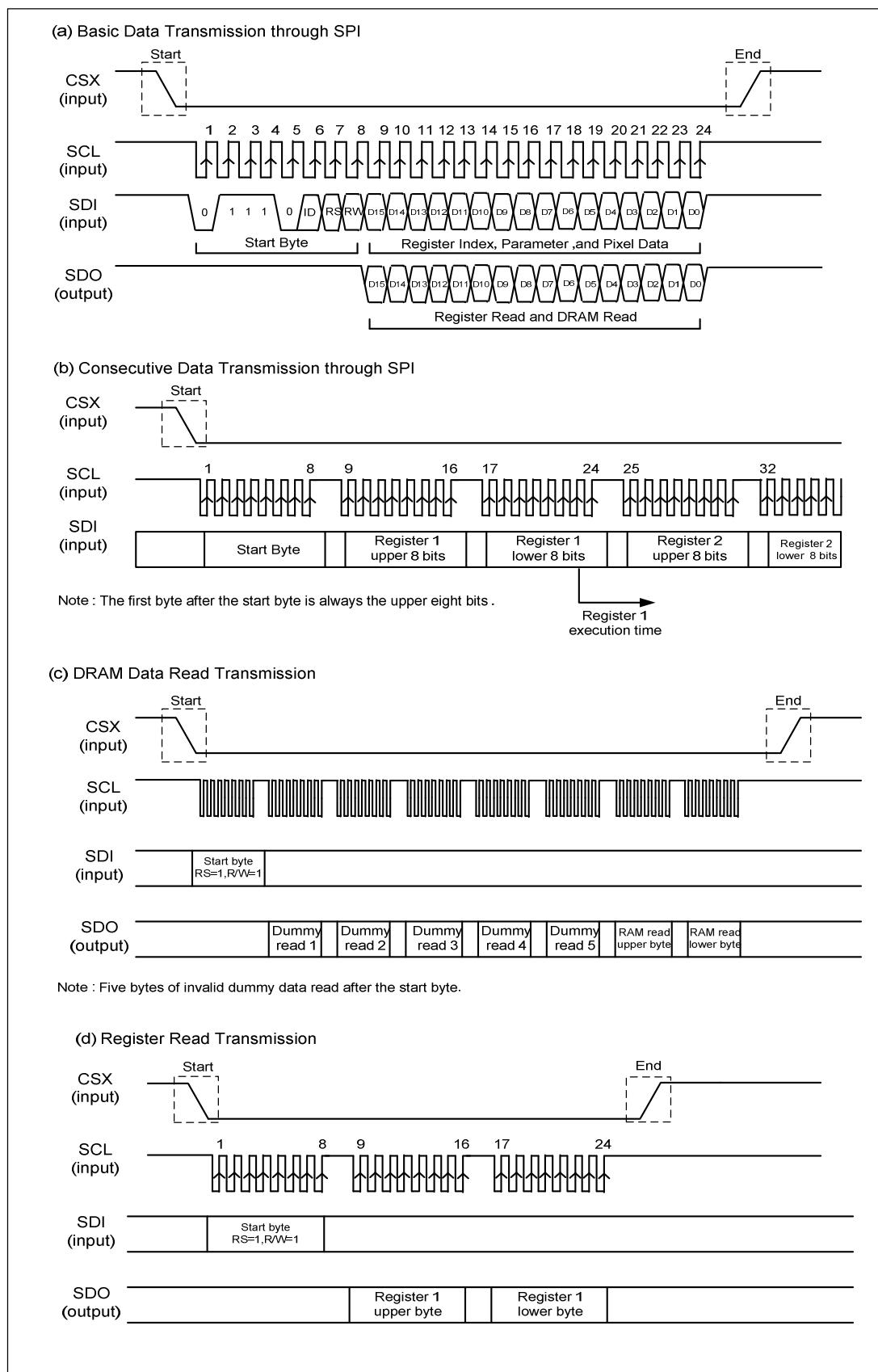
Figure 30 Data transmission through serial peripheral interface (SPI)
