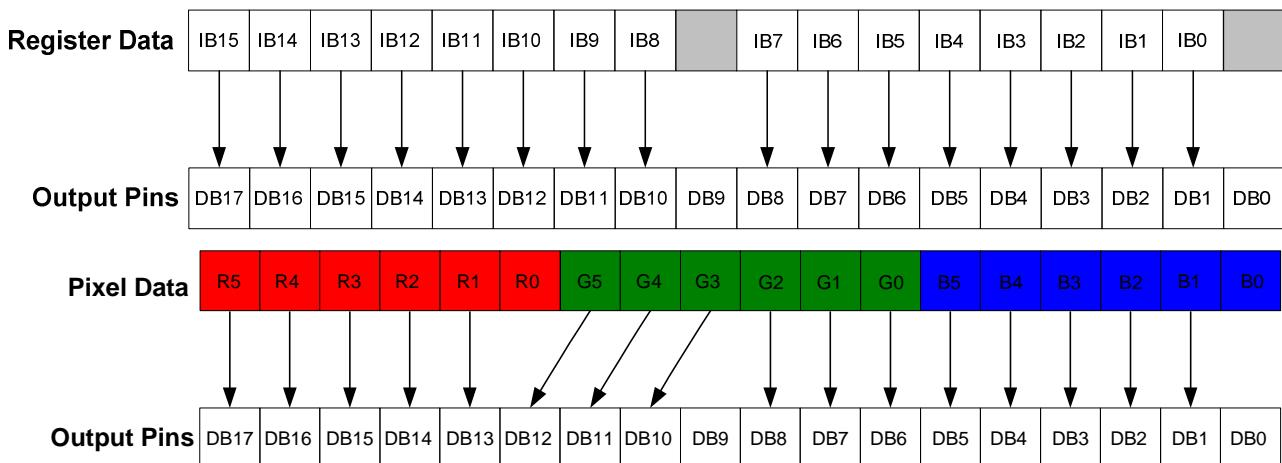
Figure 19 16-bit 8080-Series Interface Data Format (Register/Pixel Data Read)
