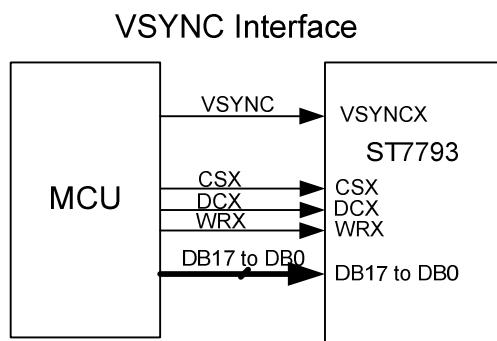
Figure 32 VSYNC Interface Connection
