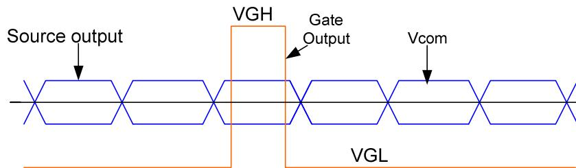
Figure 54 Voltage Output to TFT LCD Panel
