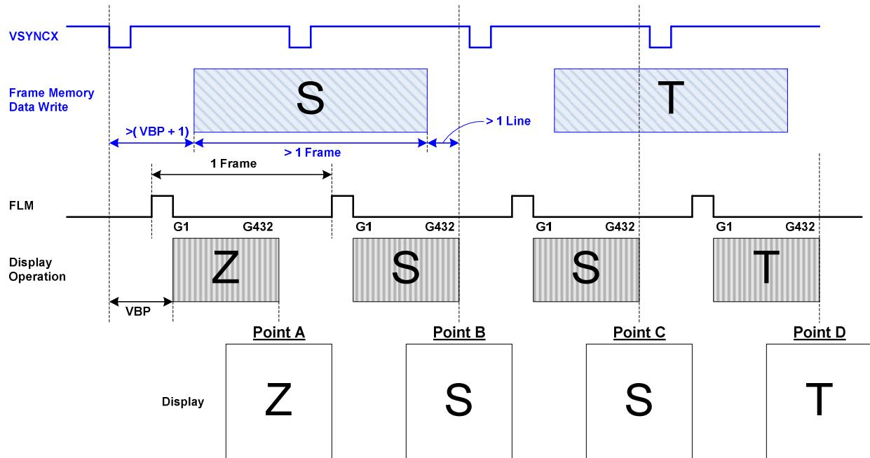
Figure 36 Operation for Lagging Mode of VSYNC Interface
