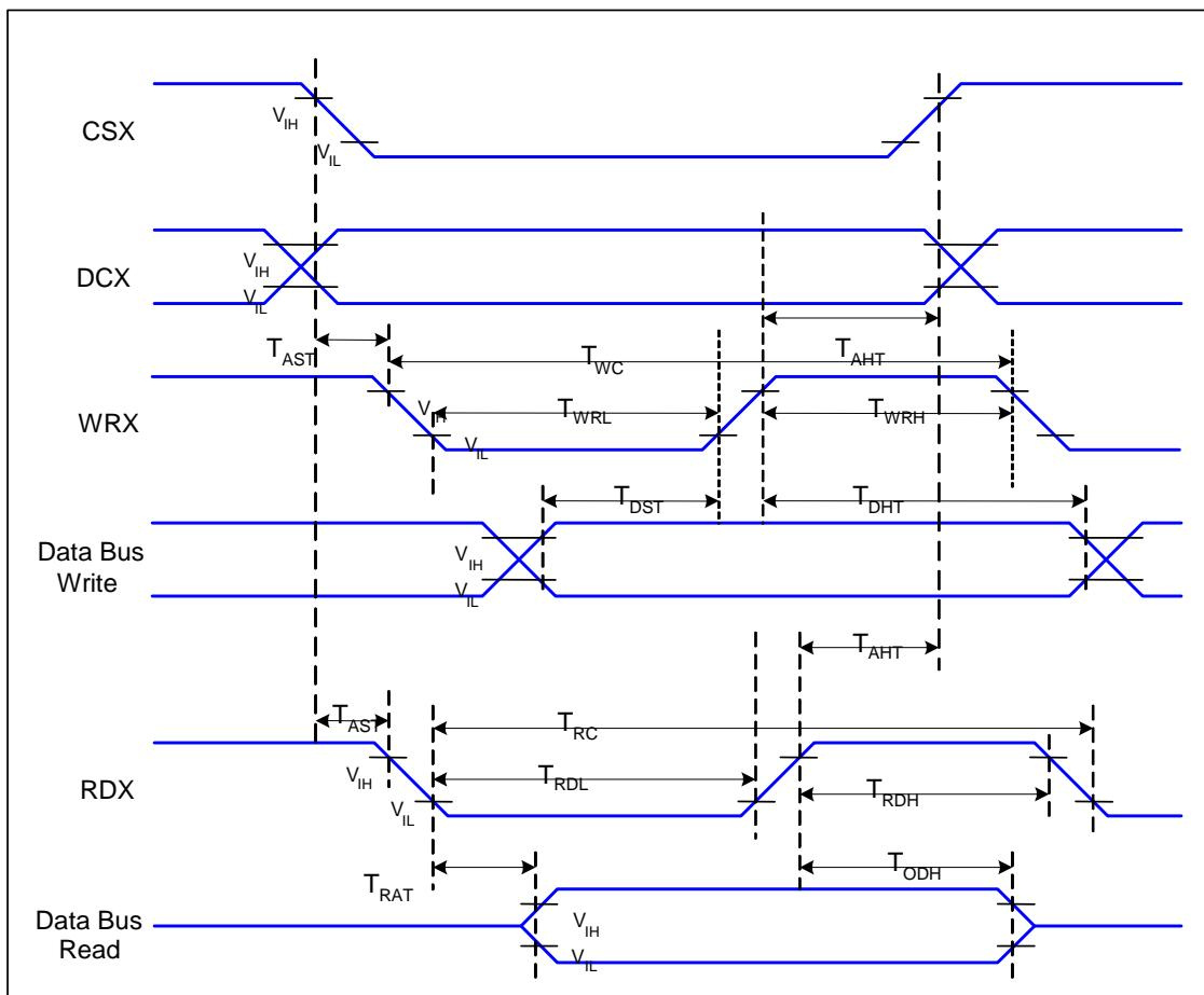
Figure 2 Parallel Interface Timing Characteristics (8080-Series MCU Interface)
