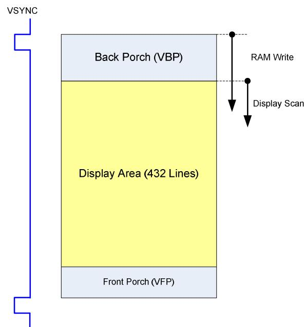
Figure 33 VSYNC Interface Operation
