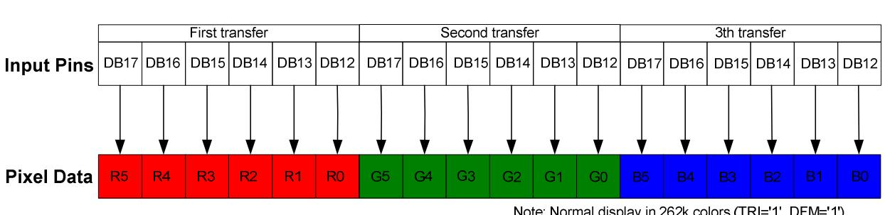
Figure 15 8-bit 8080-Series Interface Data Format (Index/Parameter/Pixel Data Write)
