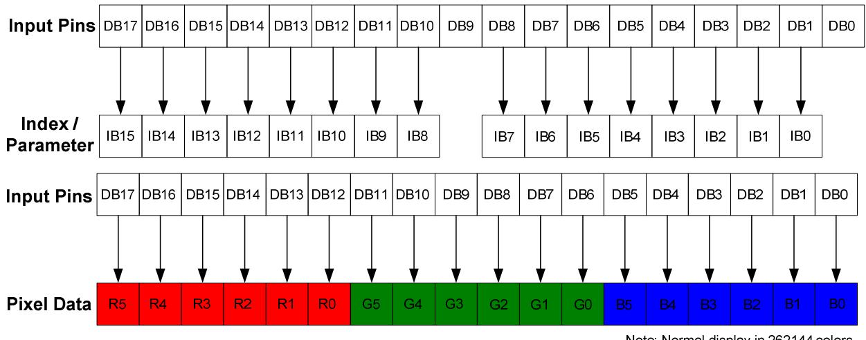
Figure 9 18-bit 8080-Series Interface Data Format (Index/Parameter/Pixel Data Write)
