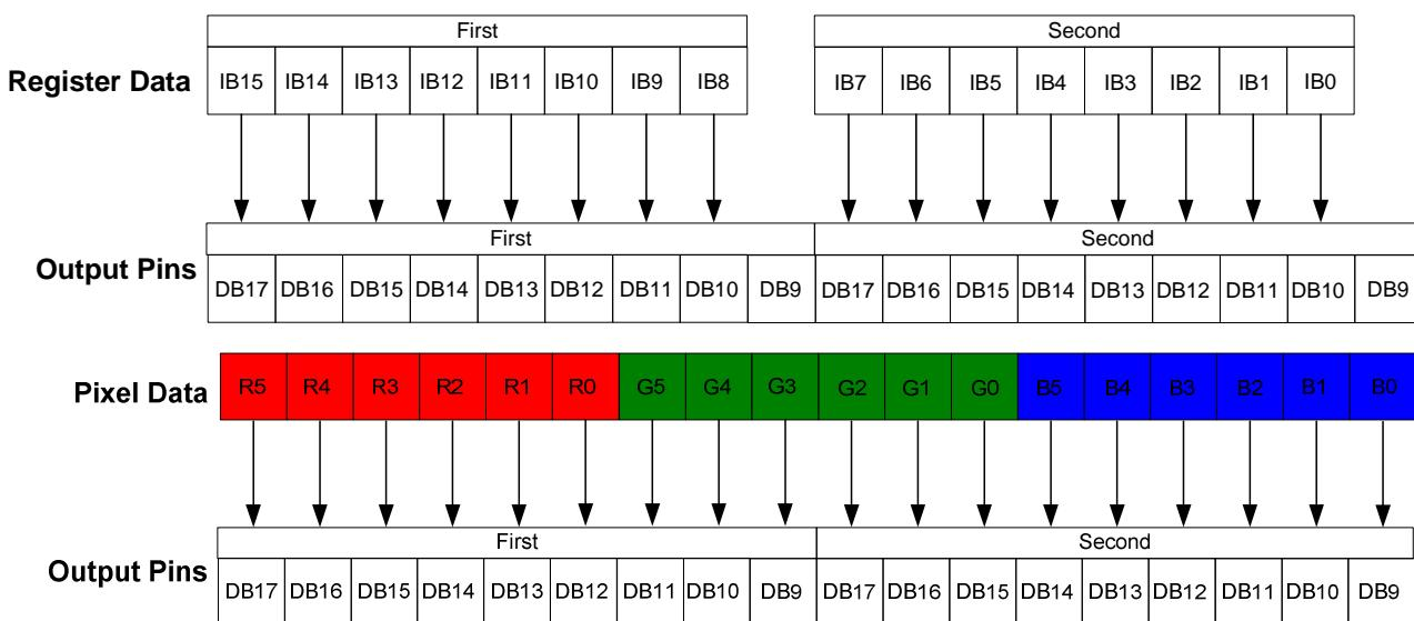
Figure 20 9-bit 8080-Series Interface Data Format (Register/Pixel Data Read)
