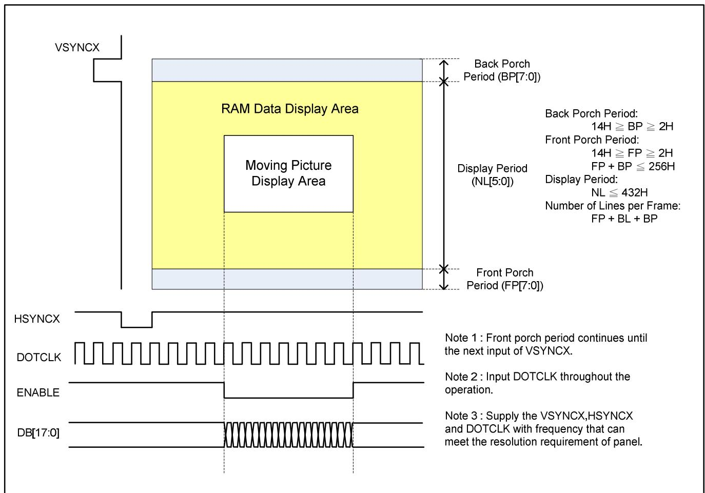
Figure 22 Display RAM Access Area via RGB Interface
