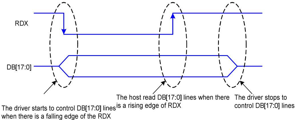
*Note1: RDX is an unsynchronized signal (It can be stopped)*
