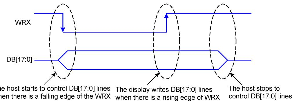
*Note: WRX is an synchronized signal (It can be stopped).*
