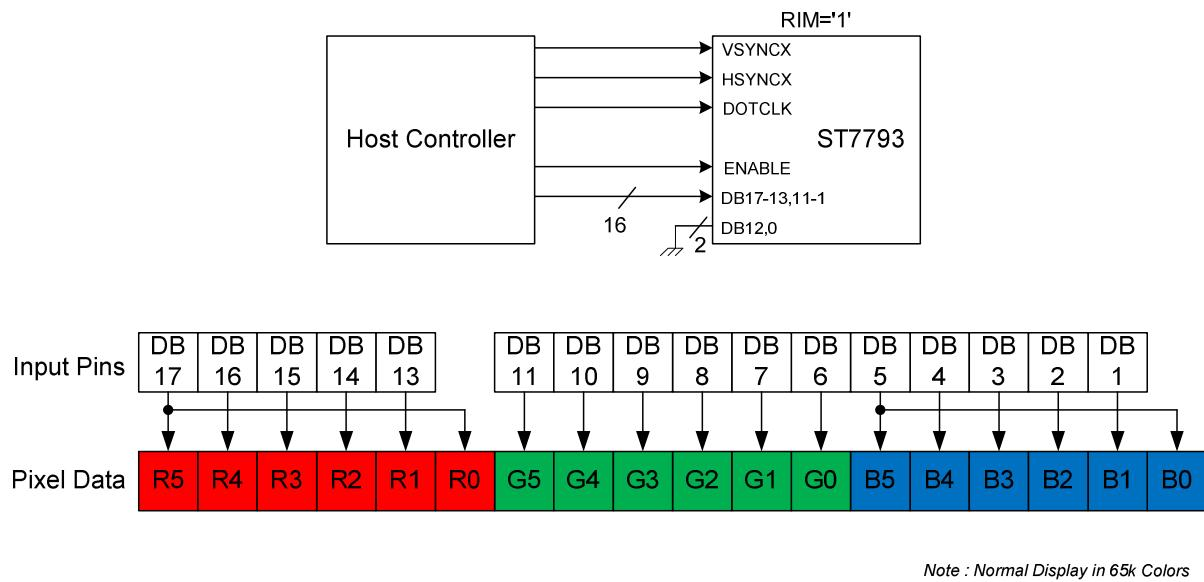
Figure 27 16-bit RGB Interface Data Format
