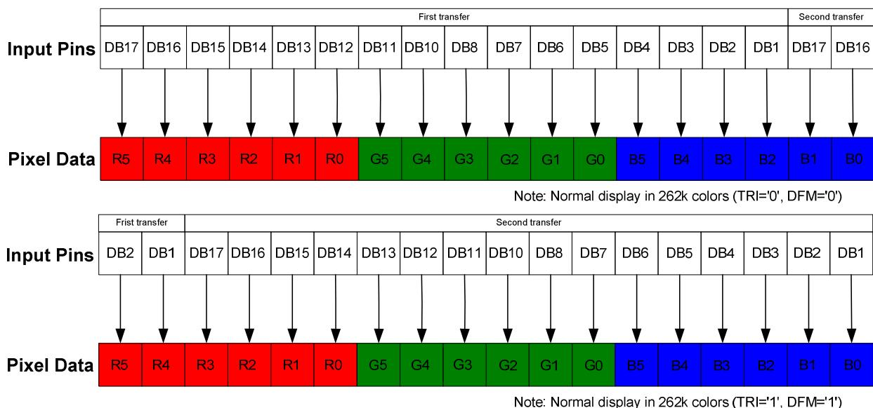
Figure 11 16-bit 8080-Series Interface Data Format (Index/Parameter/Pixel Data Write)
