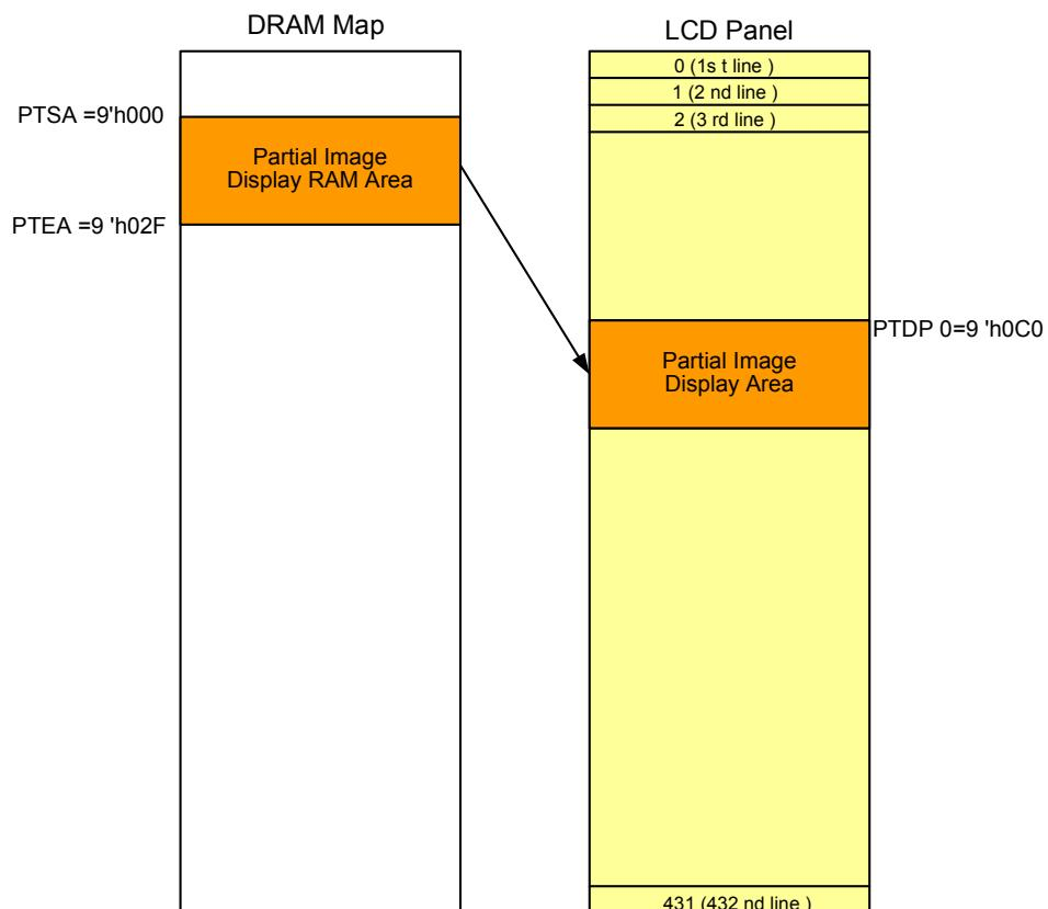
Figure 48 Partial Display Example
