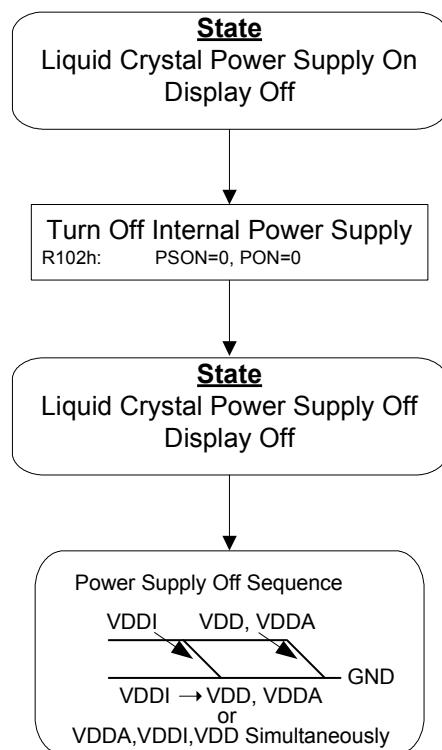
Figure 56 Power Supply Off Sequence
