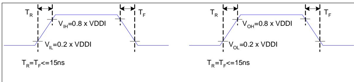
Figure 3 Rising and Falling Timing for I/O Signal
