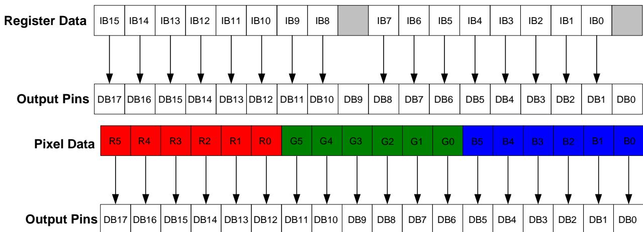
Figure 18 18-bit 8080-Series Interface Data Format (Register/Pixel Data Read)
