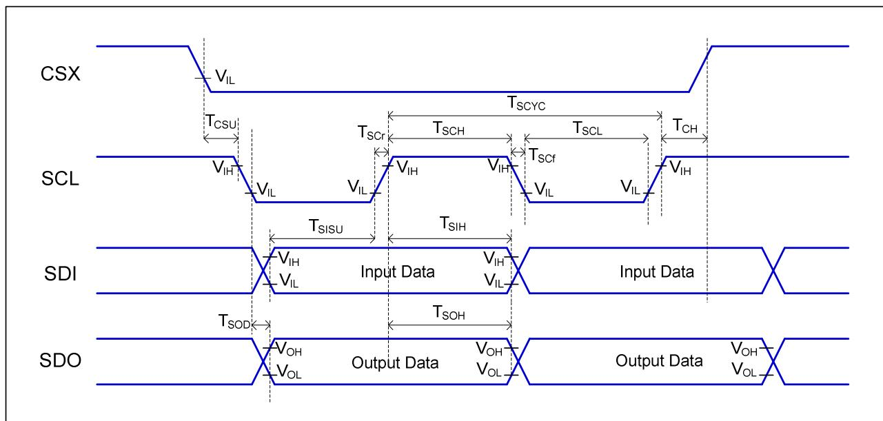
Figure 4 SPI Interface Timing Characteristics
