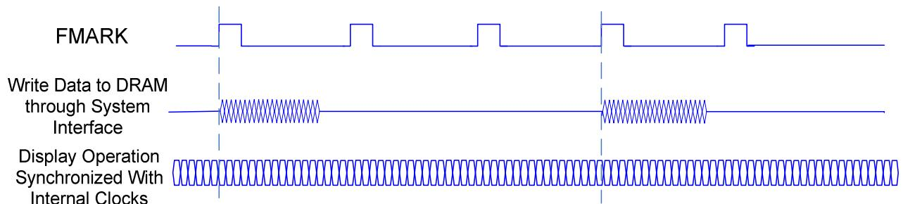
Figure 44 Moving Picture Data Transfers via FMARK Function
