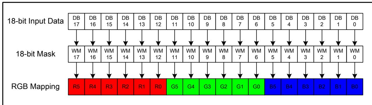
Figure 38 GRAM write with 18-bit data mask
