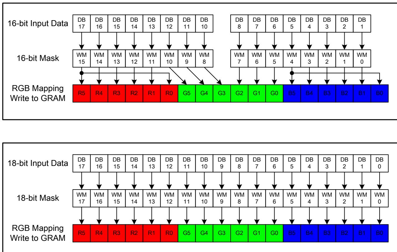
Figure 47 16-/18-bit Data Mask Function
