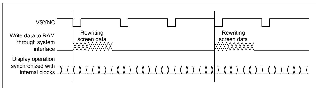
Figure11 Moving picture data transmission through VSYNC interface
