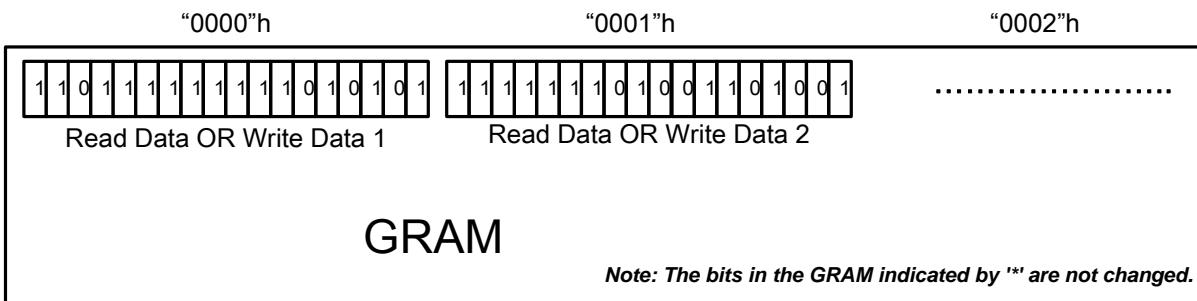
Figure 52 Write Operation of Read/Write Mode 1
