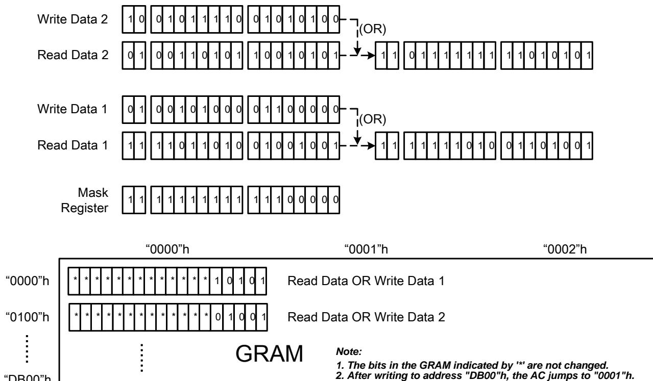
Figure 53 Write Operation of Read/Write Mode 2
