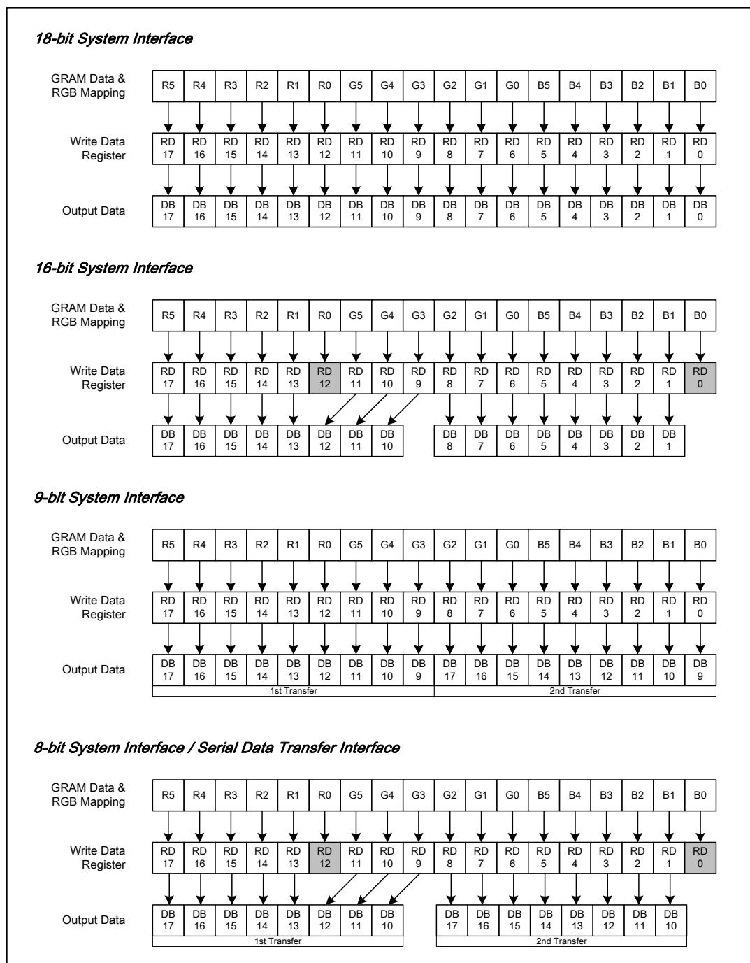
**Figure 36 Data Read from GRAM through Read Data Register in 18-/16-/9-/8-bit Interface Mode**
