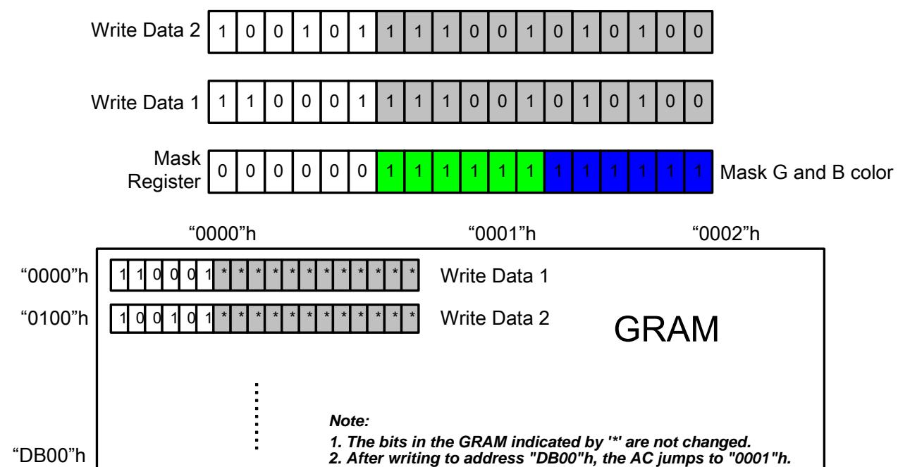
Figure 49 Write Operation of Write Mode 2
