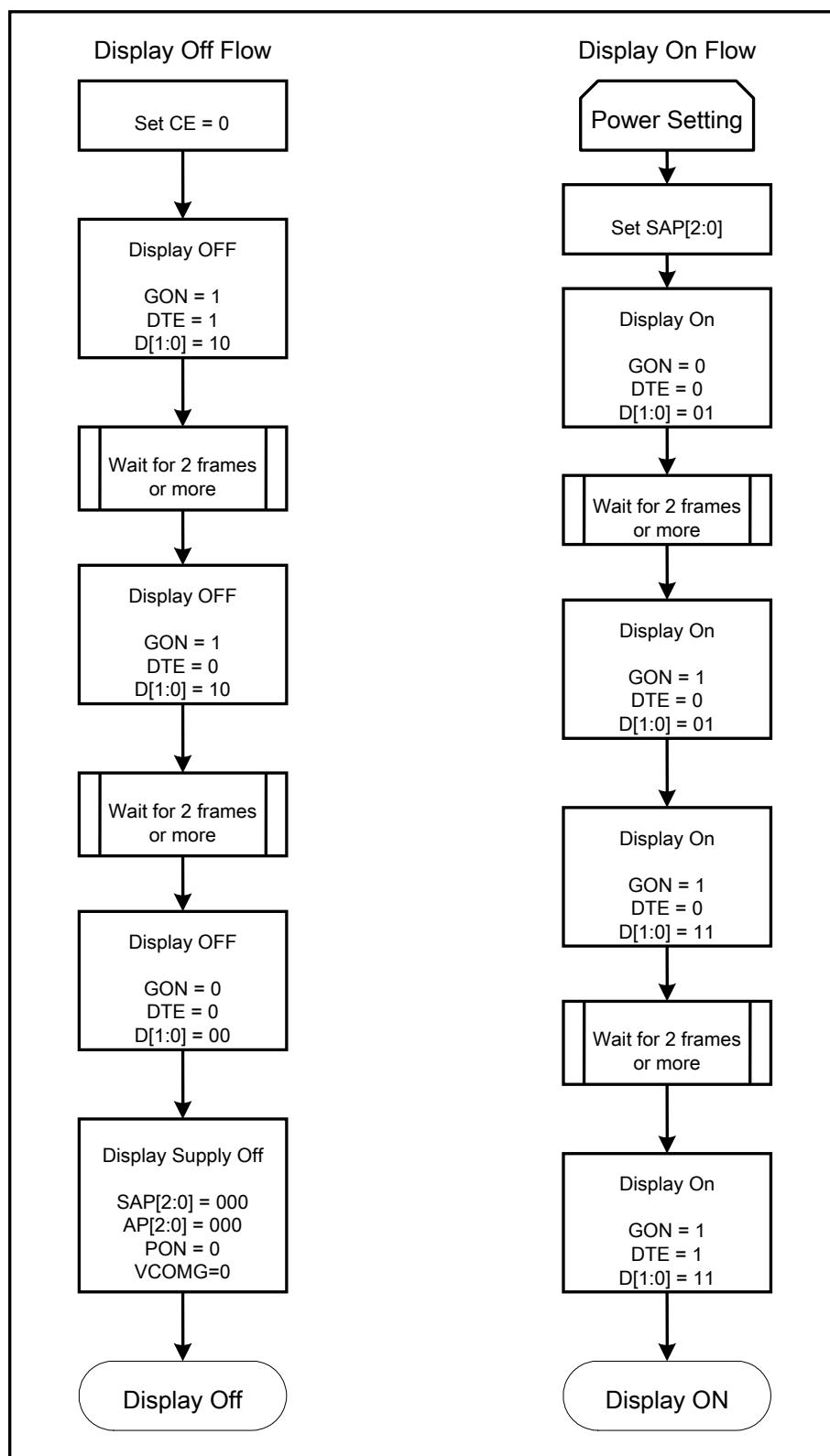
Figure 63 Display On/Off Register Setting Sequence
