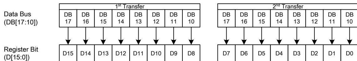
**Figure23 Register setting with i80/M68 System Interface**
