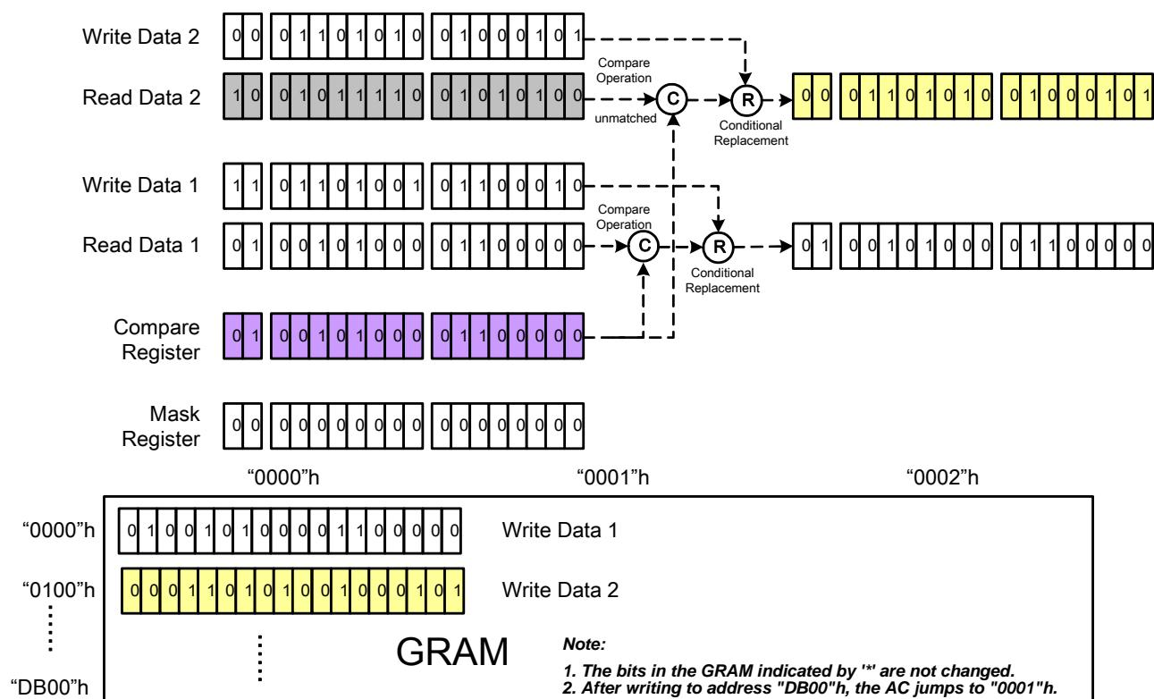
Figure 55 Write Operation of Read/Write Mode 4
