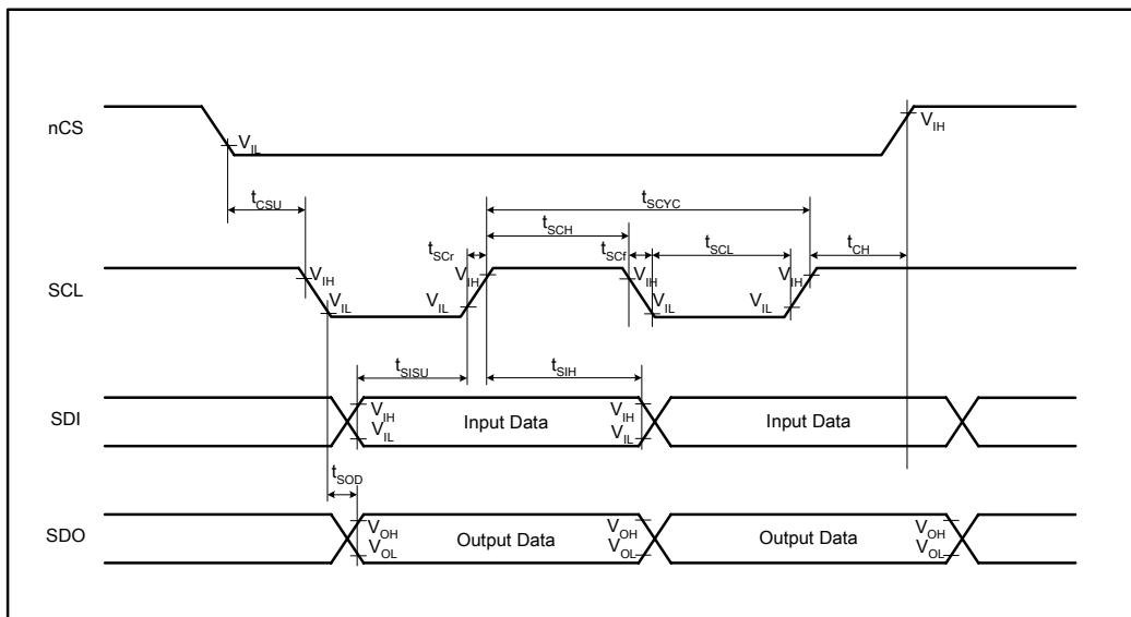
Figure 75 SPI System Bus Timing
