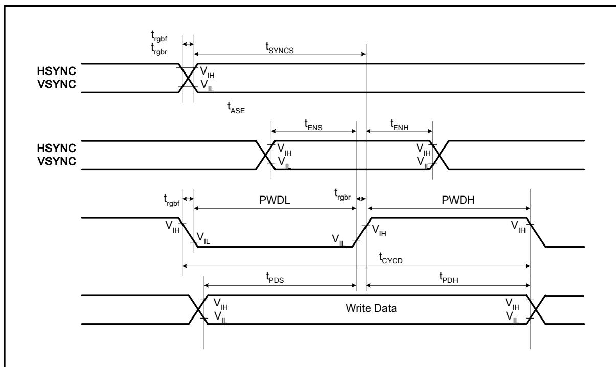
Figure76 RGB Interface Timing
