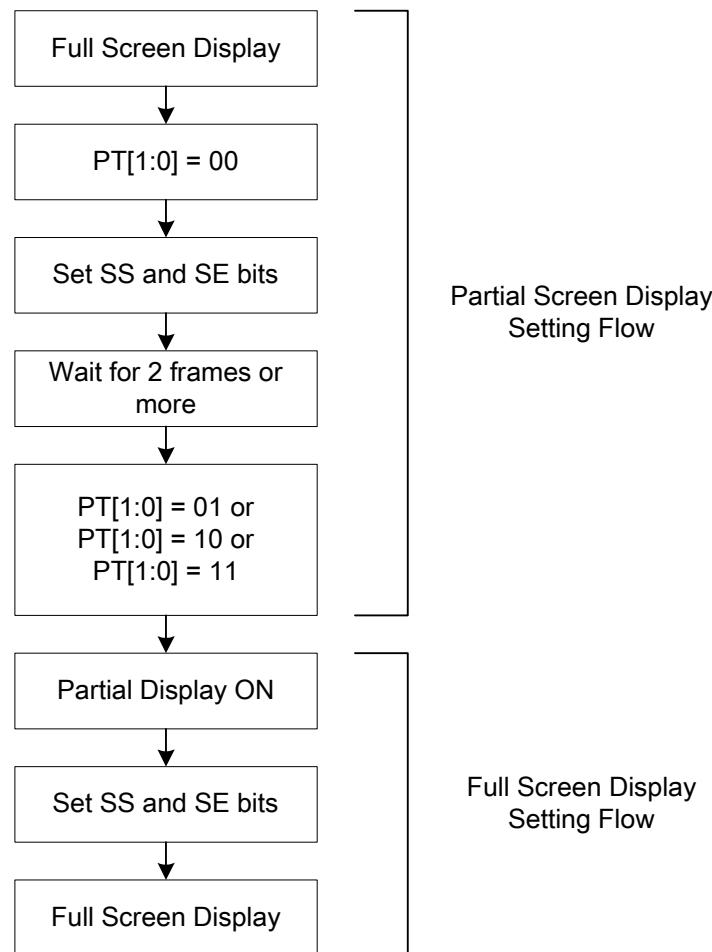
**Figure 70 Partial Display Setting Flow**
