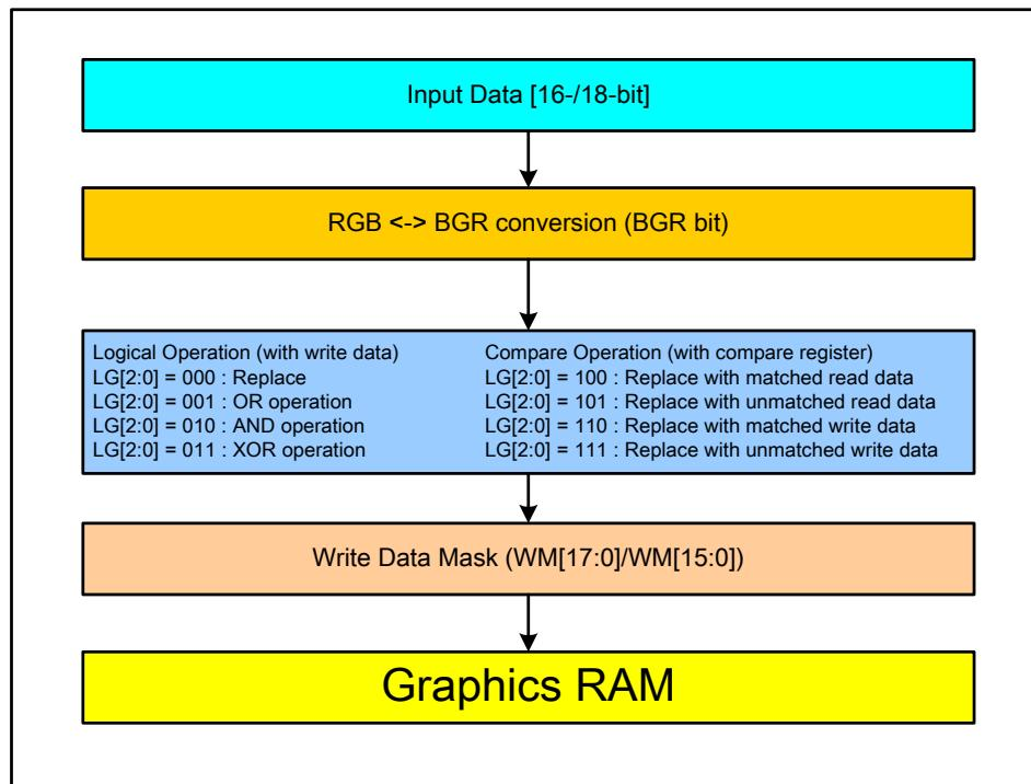
Figure31 Data Operation with Mask and Compare Function
