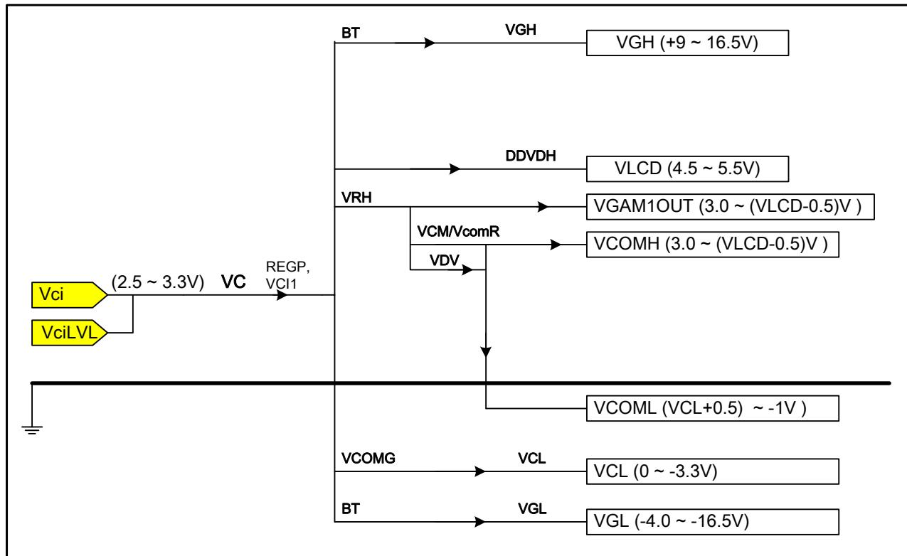
**Figure 66 Voltage Configuration Diagram**
