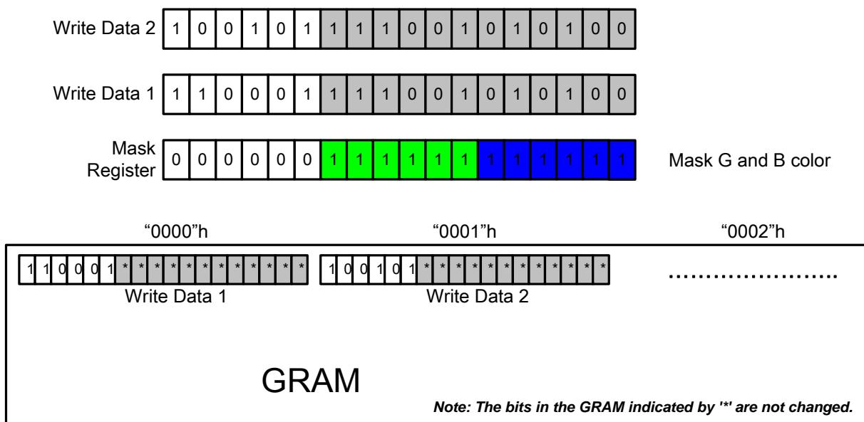
**Figure 48 Write Operation of Write Mode 1**
