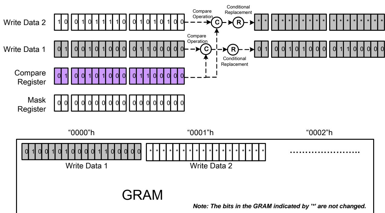
Figure 50 Write Operation of Write Mode 3
