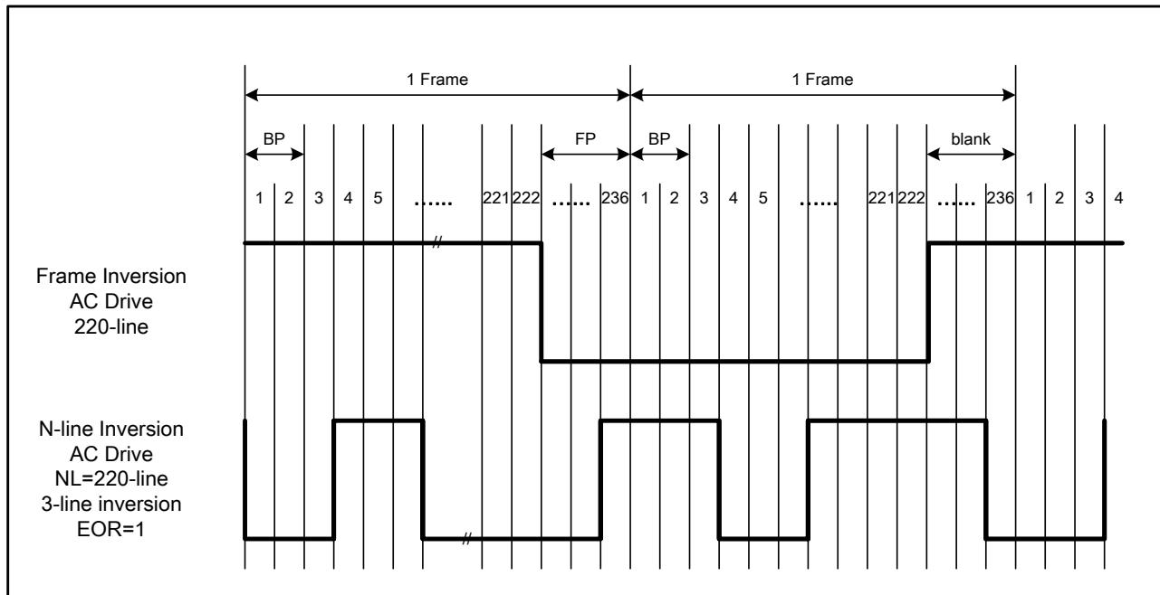
**Figure 26 n-line Inversion AC Drive**
