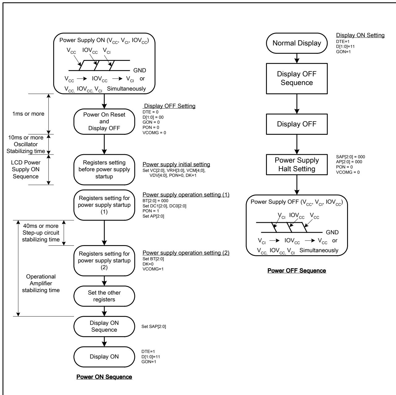
Figure 65 Power Supply ON/OFF Sequence
