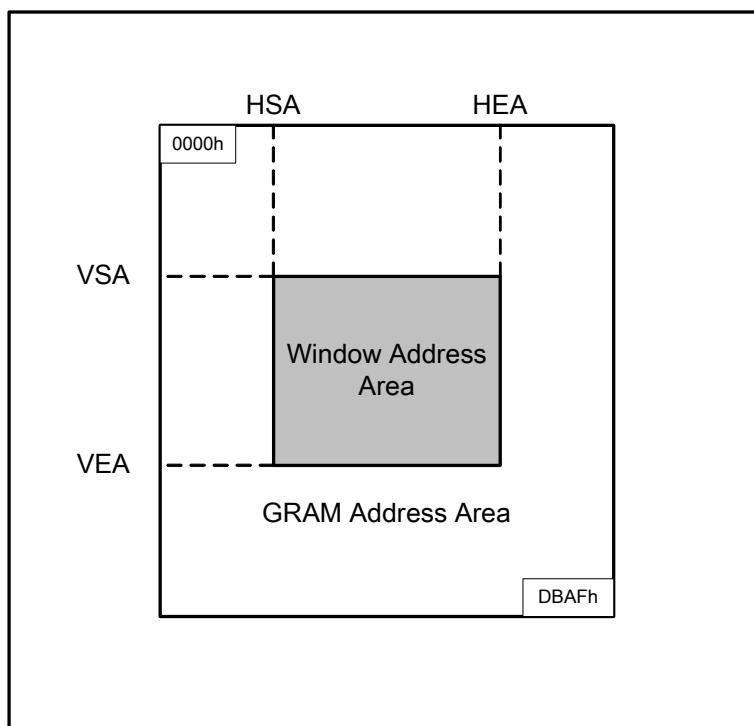
Figure 41 GRAM Access Range configuration
