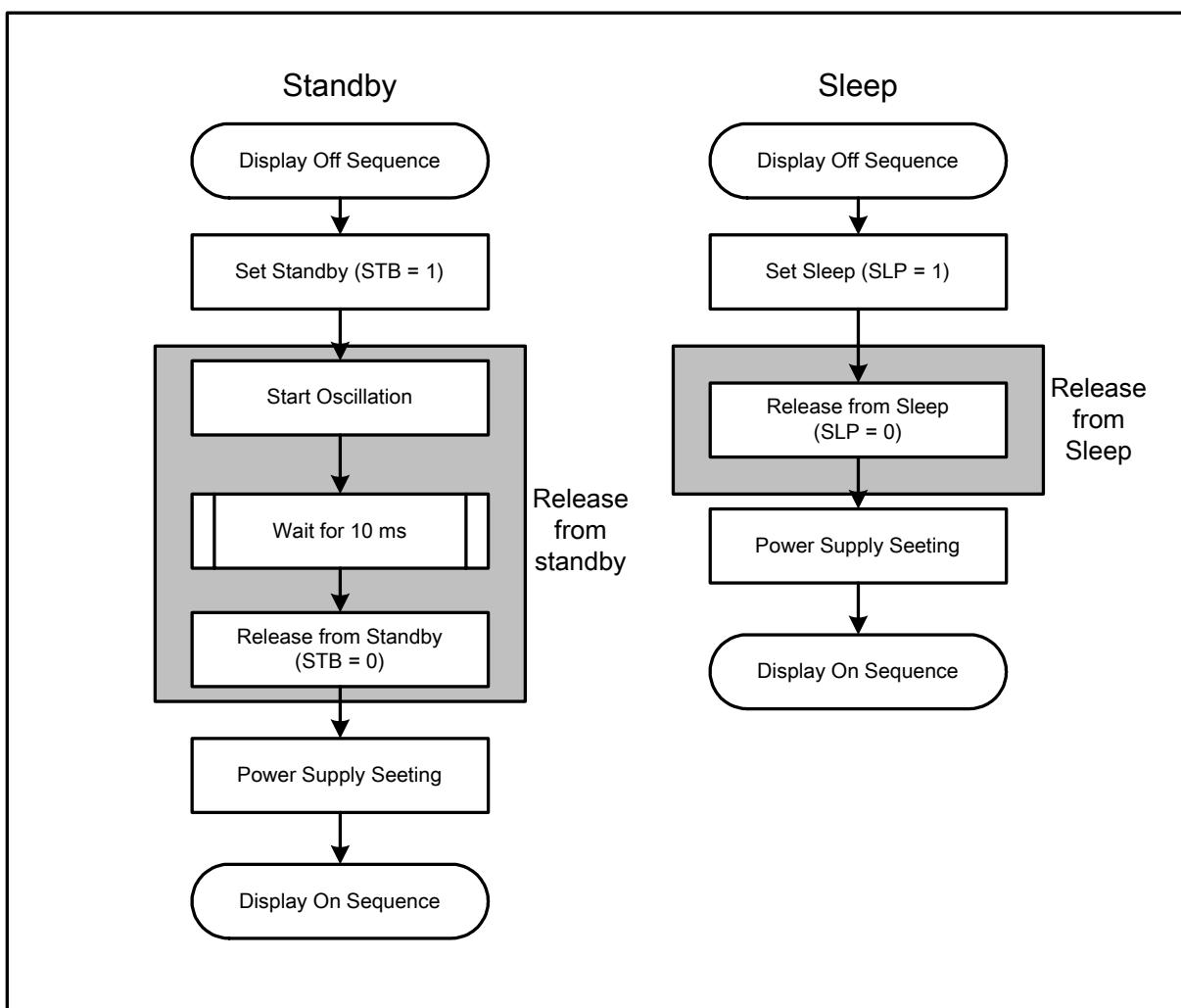
Figure 64 Standby/Sleep Mode Register Setting Sequence
