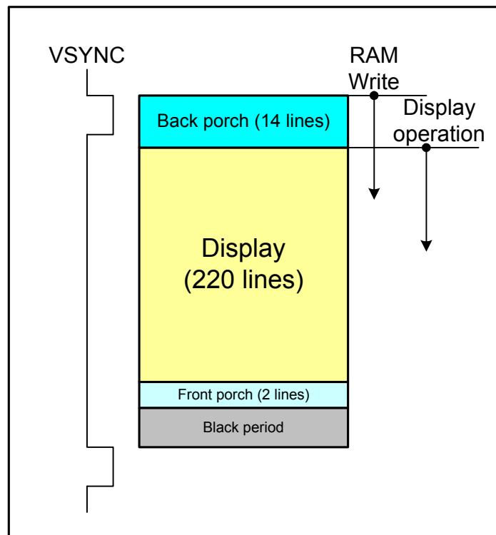
**Figure12 Operation through VSYNC Interface**
