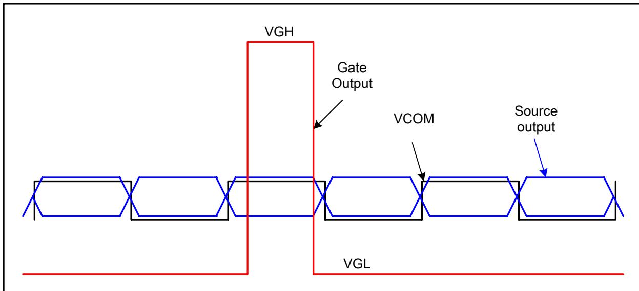
Figure 67 Voltage Output to TFT LCD Panel
