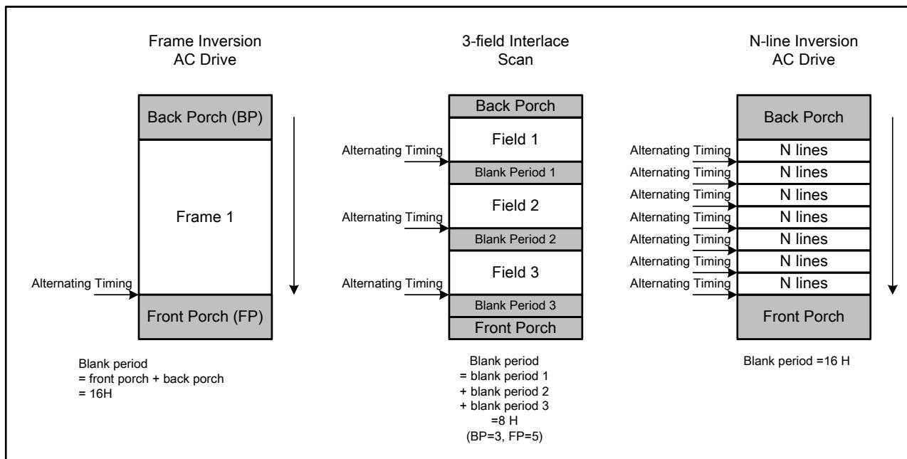
Figure29 AC Driving Alternating Timing
