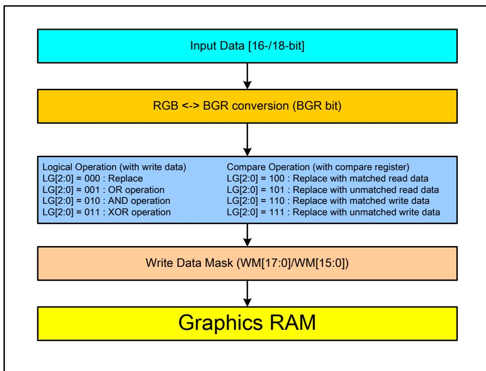
Figure35 Data Operation with Mask and Compare Function
