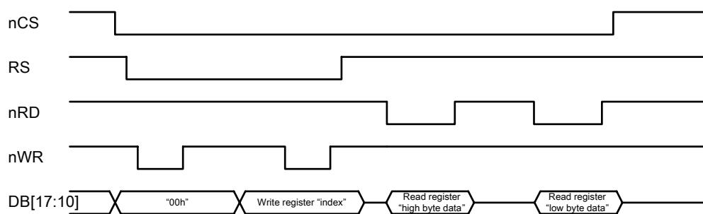
**Figure 24 Register Read/Write Timing of i80 System Interface**
