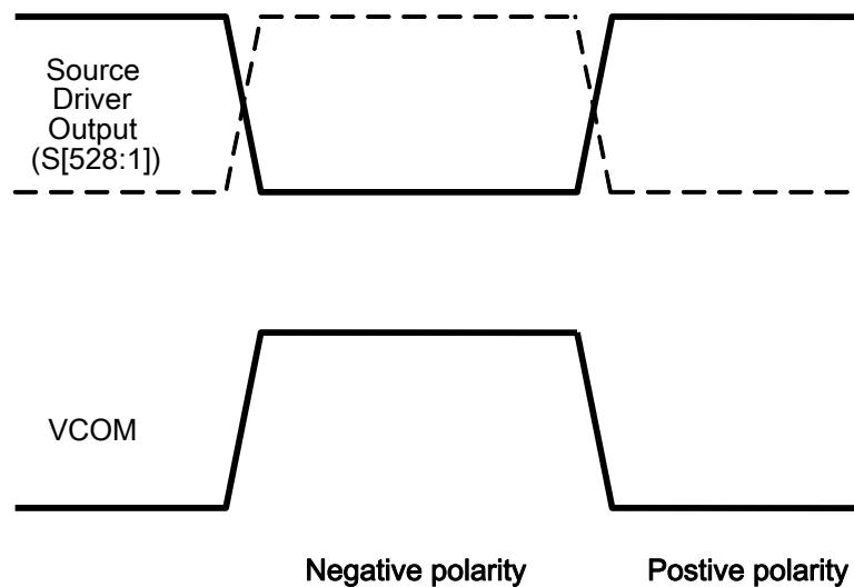
**Figure 60 Relationship between Source Output and VCOM**
