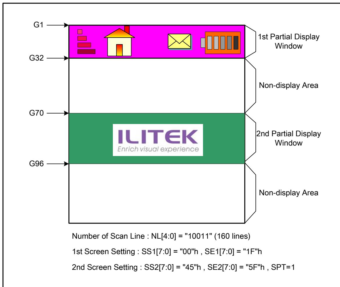
**Figure 69 Partial Display Example**
