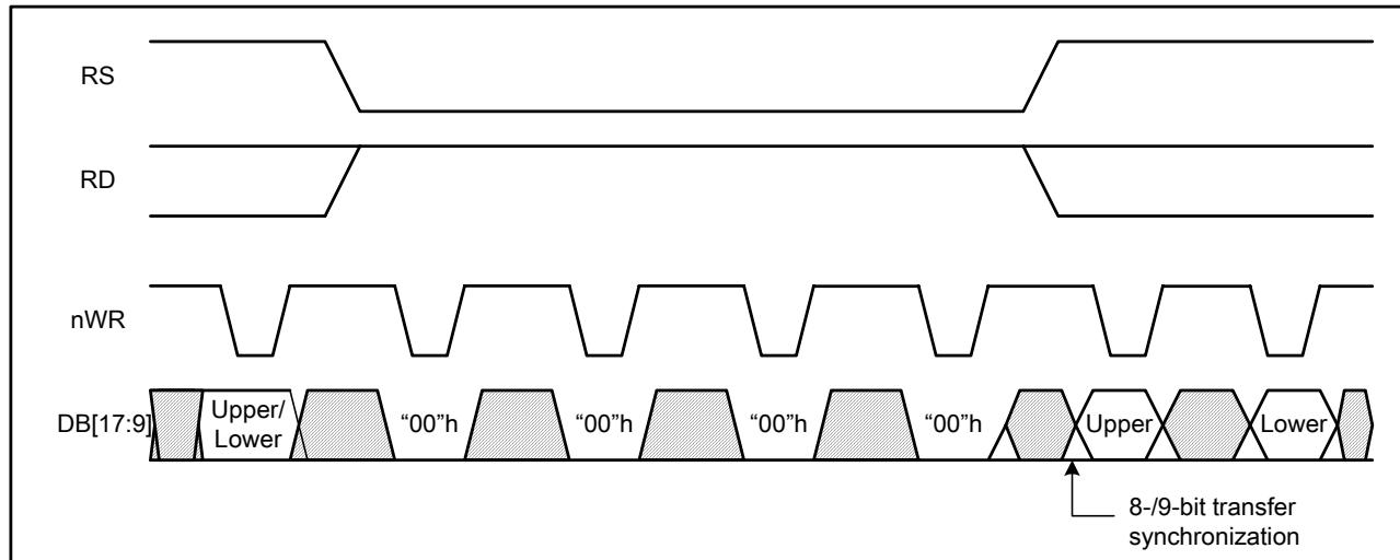
Figure6 Data Transfer Synchronization in 8/9-bit System Interface
