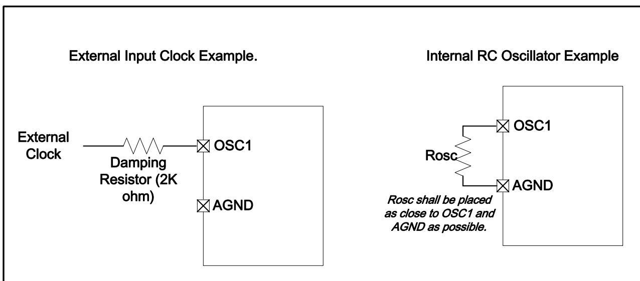
Figure 68 Oscillation Connection
