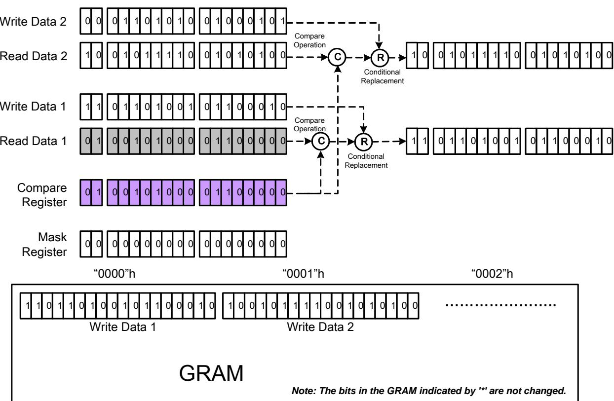
Figure 54 Write Operation of Read/Write Mode 3
