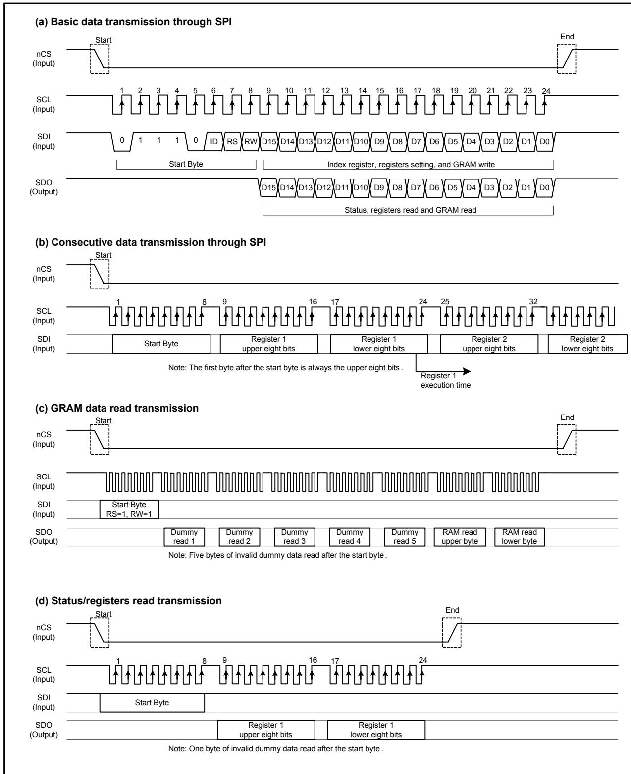
**Figure8 Data transmission through serial peripheral interface (SPI)**
