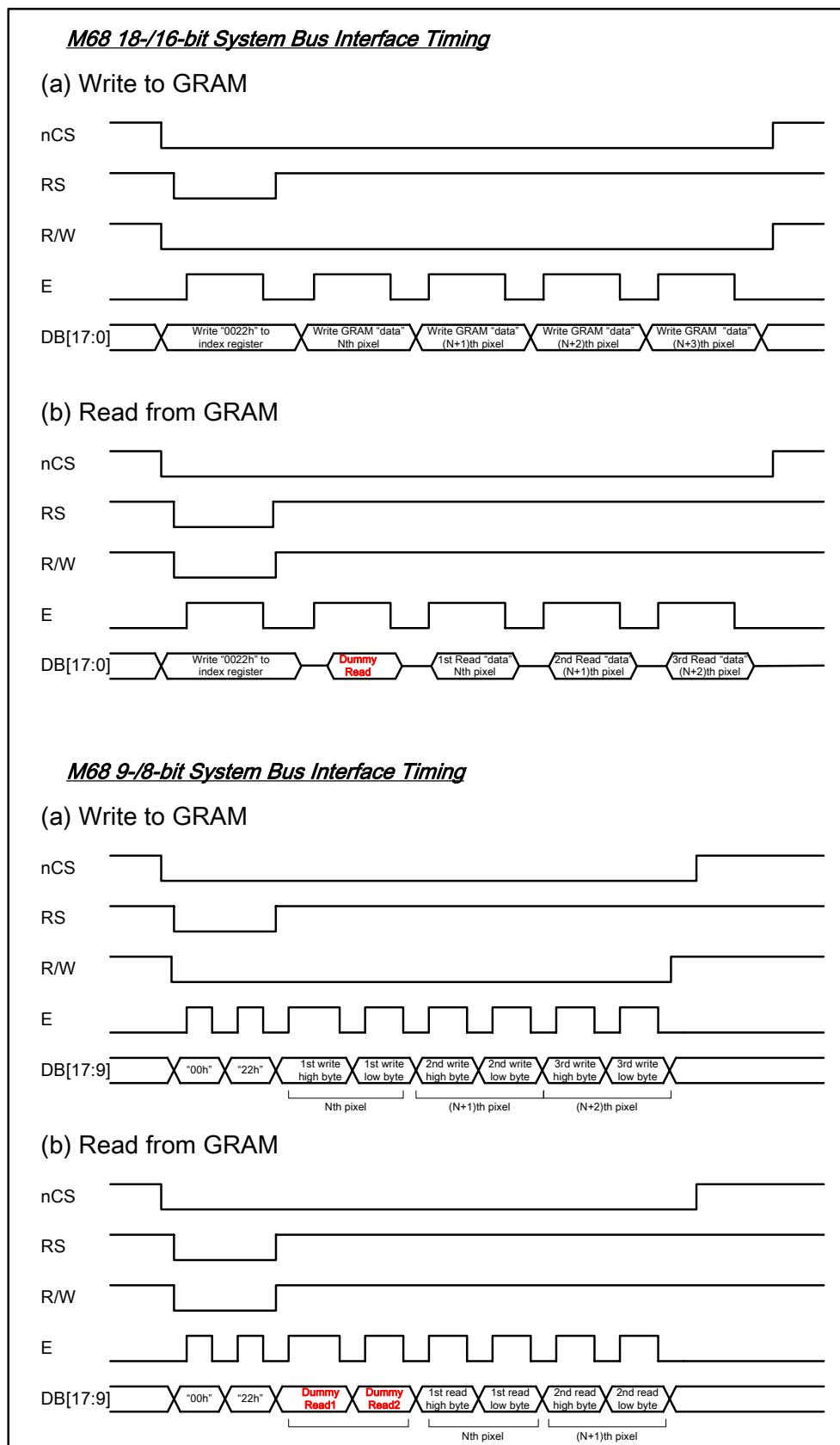
**Figure 43 GRAM Read/Write Timing of M68-System Interface**
