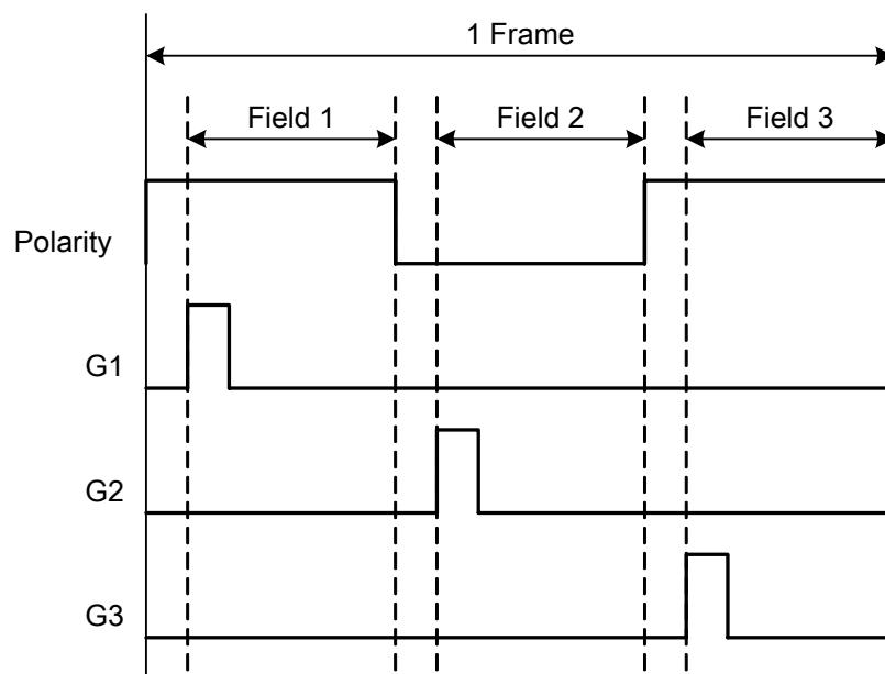
Figure28 Output Timing of Interlace Gate Signals (Three-field is selected)
