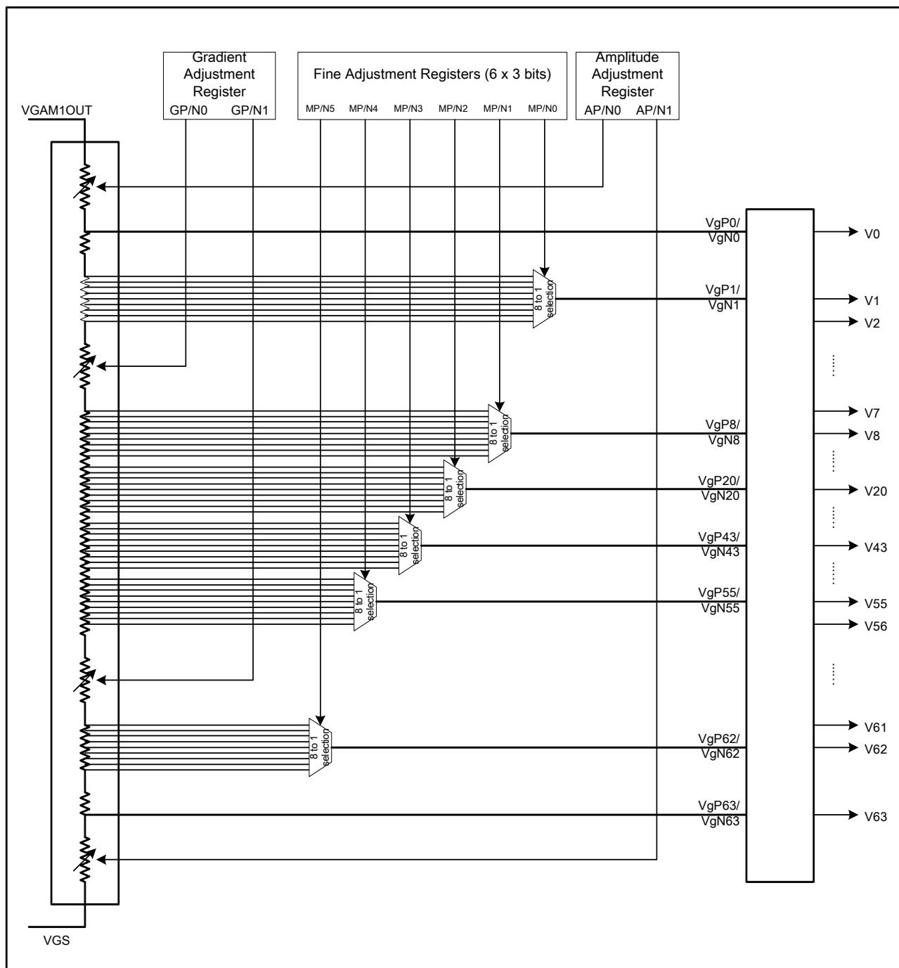
Figure 57 Grayscale Voltage Generation
