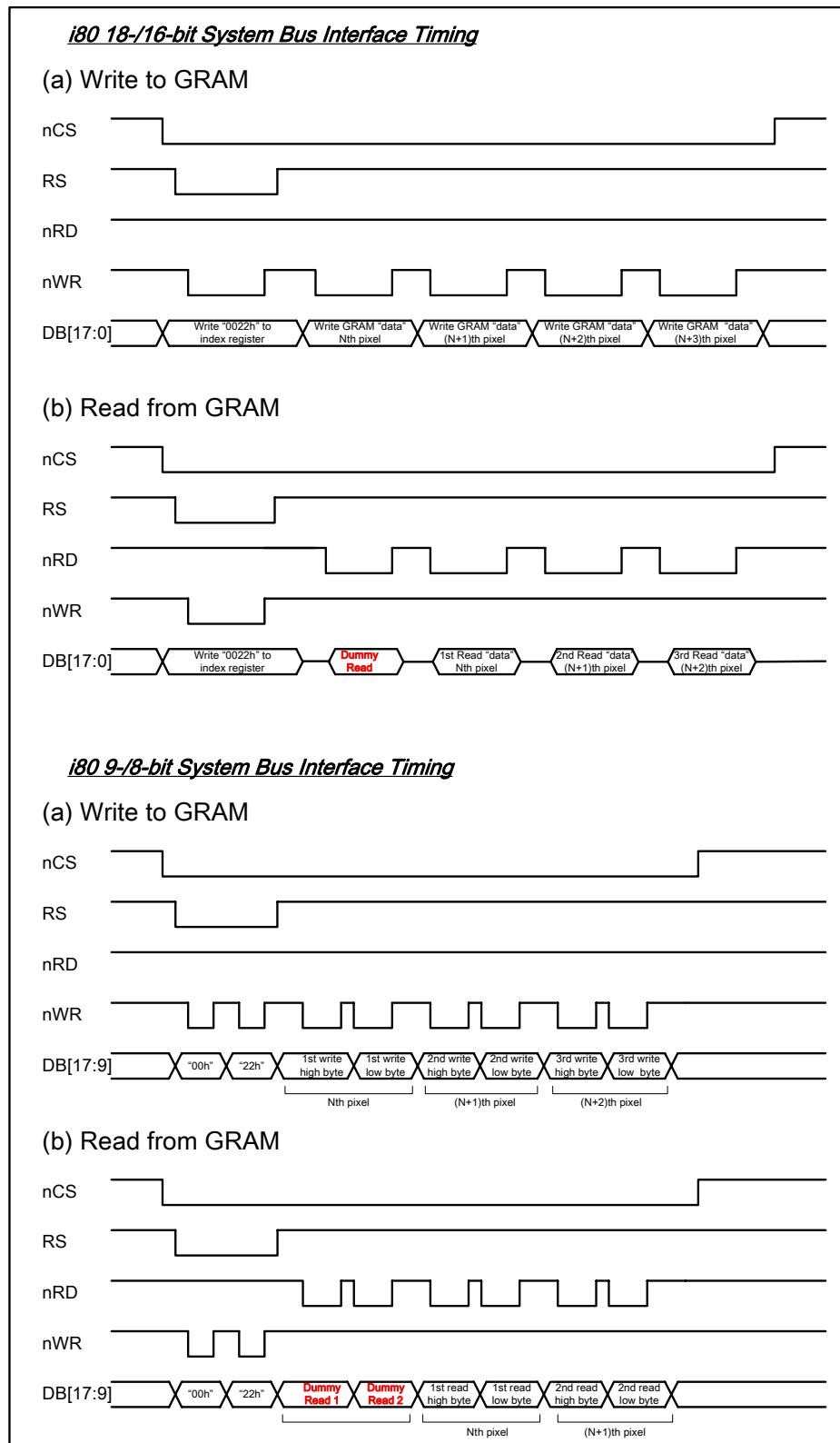
Figure42 GRAM Read/Write Timing of i80-System Interface
