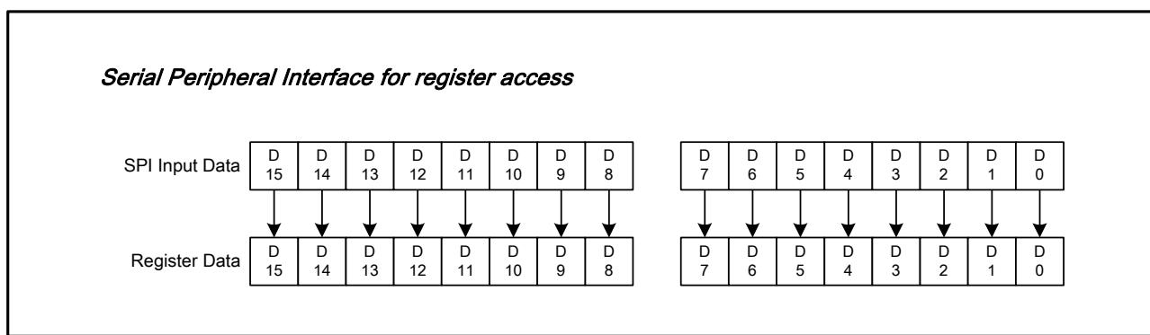
Figure22 Register Setting with Serial Peripheral Interface (SPI)
