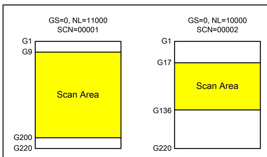
Figure 40 Scanning Start Position for Gate Driver
