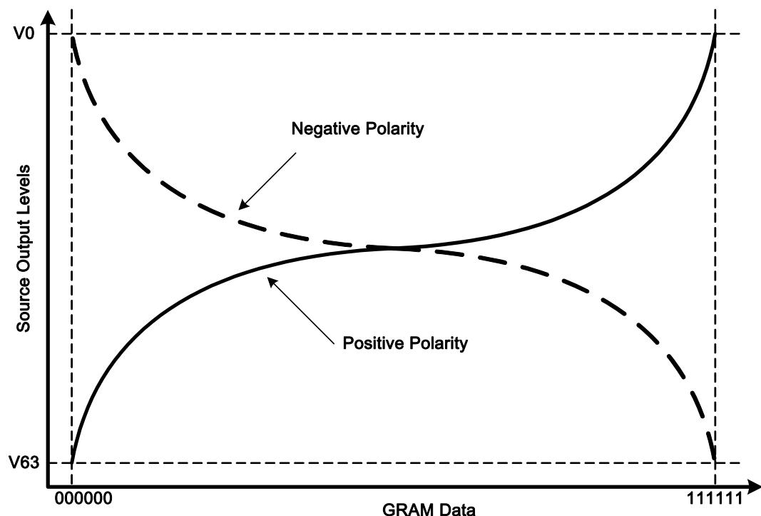
**Figure 61 Relationship between GRAM Data and Output Level**
