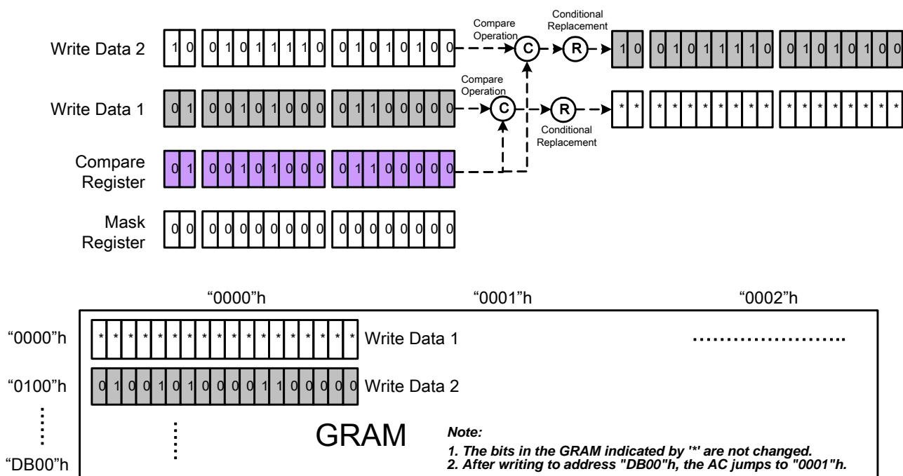
**Figure 51 Write Operation of Write Mode 4**
