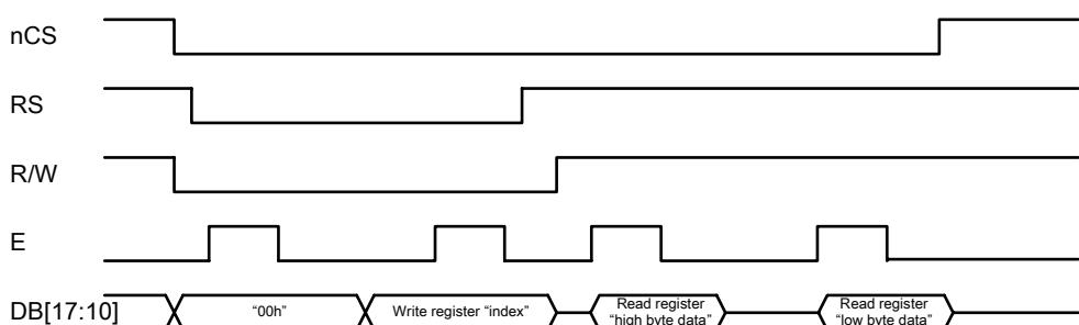
**Figure 25 Register Read/Write Timing of M68 System Interface**
