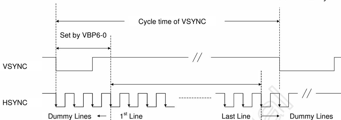
Figure 2.17 No. of clock cycle of HSYNC
