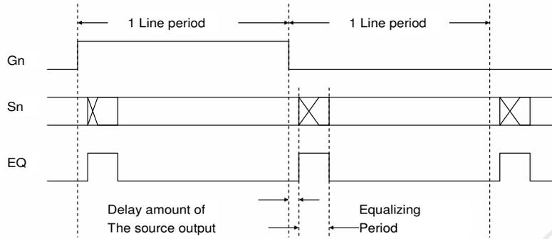
Figure 2.10 EQ timing diagram
