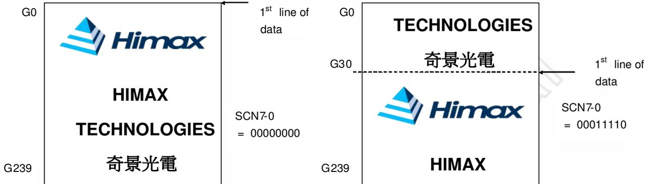
Figure 2.14 Gate scan display position
