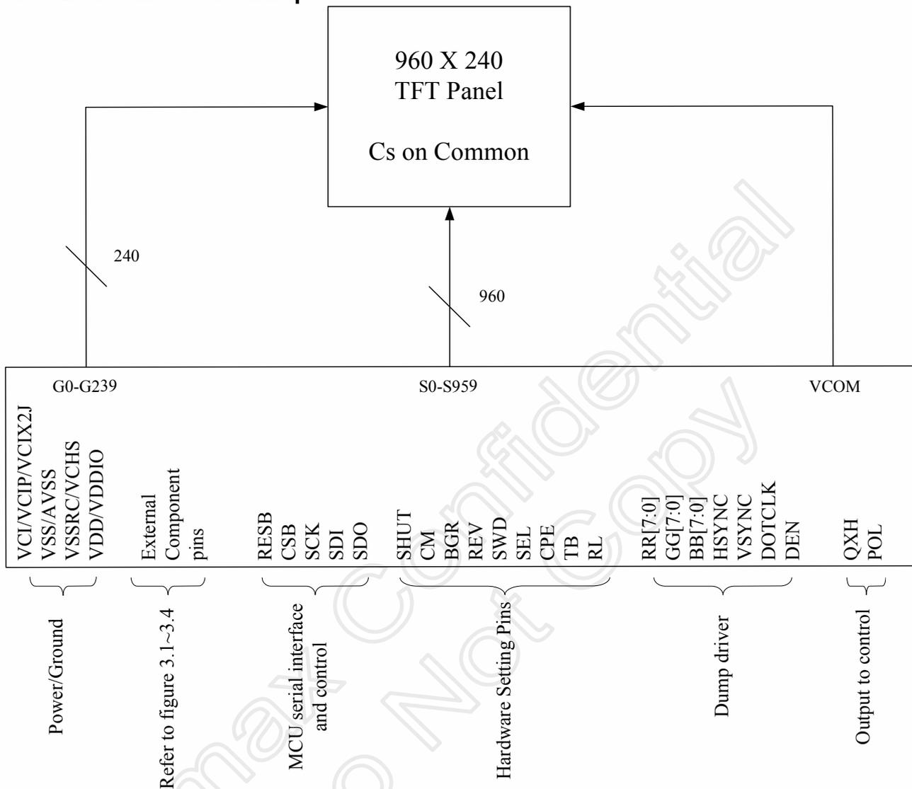
Figure 3.6 Panel connection example.
