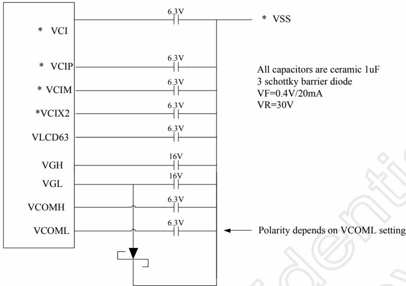
Figure 3.4 Filtering and charge sharing capacitors
