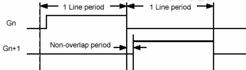
Figure 2.9 NO timing diagram
