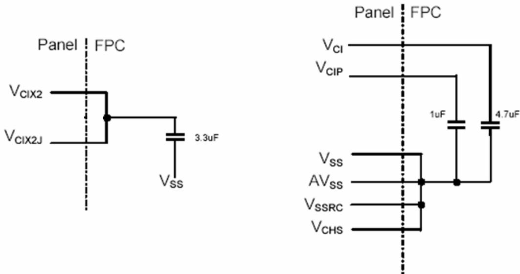
Figure 3.5 Panel and FPC connection
