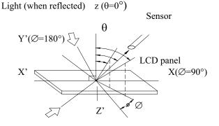
Light (when transmitted )  $Y(\varnothing=0^{\circ})$   $(\theta=90^{\circ})$
