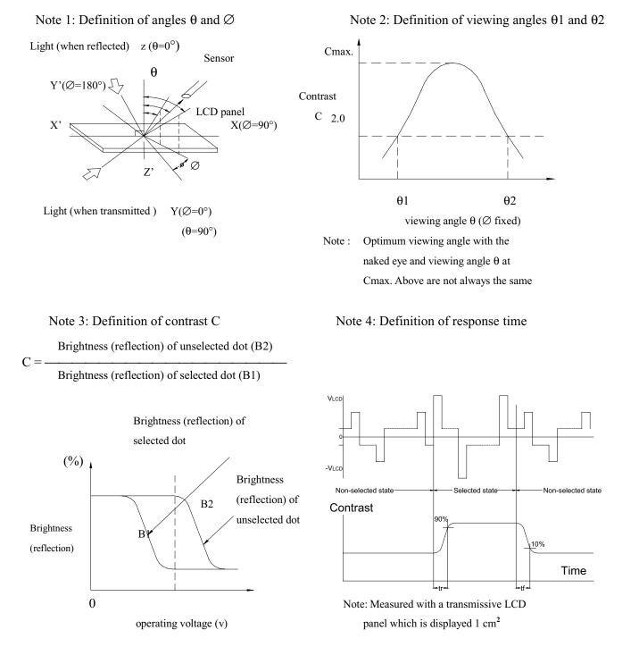
$V_{LCD}$ : Operating voltagef<sub>FRM</sub>: Frame frequency t<sub>r</sub> : Response time (rise) t<sub>f</sub>: Response time (fall)
