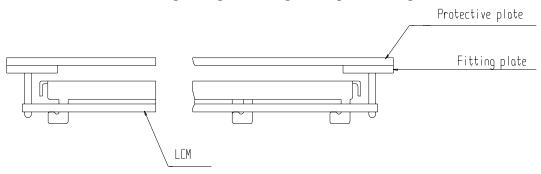
(2) When assembling the LCM into other equipment, the spacer to the bit between the LCM and the fitting plate should have enough height to avoid causing stress to the module surface, refer to the individual specifications for measurements. The measurement tolerance should be  $\pm 0.1 \, \text{mm}$ .
