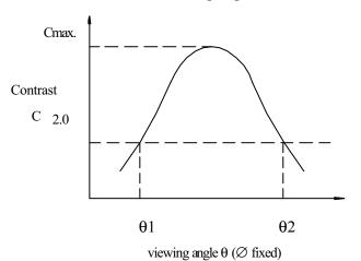
Note : Optimum viewing angle with the naked eye and viewing angle  $\theta$  at Cmax. Above are not always the same
