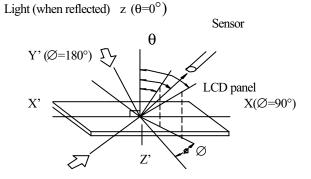
Light (when transmitted )  $Y(\varnothing=0^{\circ})$   $(\theta=90^{\circ})$
