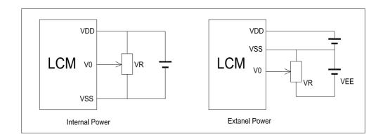
$V_{DD^{\sim}}V_0\text{: LCD Driving voltage}$
