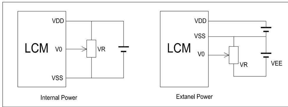
$V_{DD}-V_0$ : LCD Driving voltage
