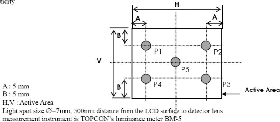
FIG. 3 The definition of viewing angle
