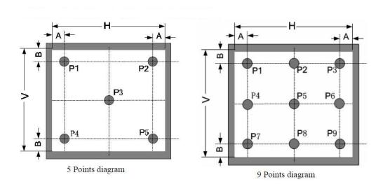
Fig2 Note1 For TFT Module Test point:9 points( as 9 Points diagram )
