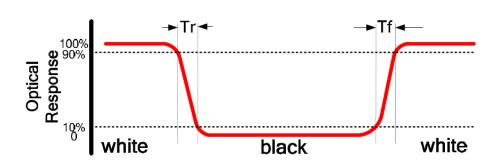
FIG.1. Measuring method for Contrast ratio, surface luminance, Luminance uniformity, CIE (x, y) chromaticity
