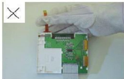
Please don't stretch interface of output, such as FPC cable.
