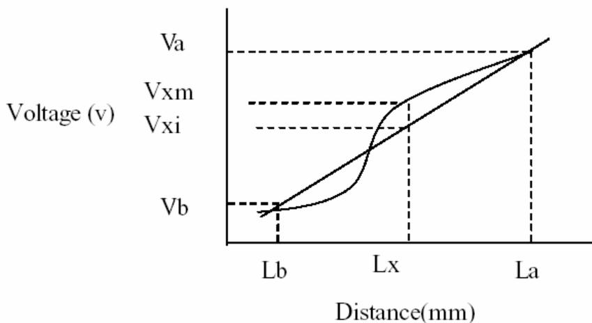
$$\text{Linearity} = \frac{|V_{xi} - V_{xm}|}{(V_a - V_b)} * 100\%$$
