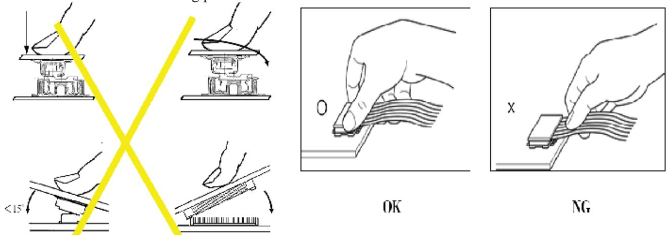
**Precaution for soldering to the LCM**
