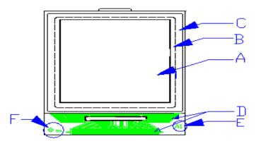
A: active area (A.A); B: visible area (V.A); C: non-visible area; D: electrode; E: special marker; F: Right S;
