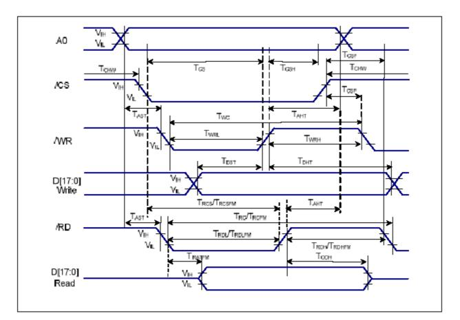
(VSS=0V, VDDI=1.65V to 2.9V, VDDA=2.3V to 3.3V, Ta = -30 to 70 · €)
