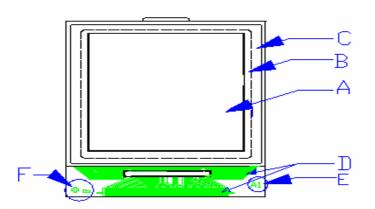
A: active area (A.A); B: visible area (V.A); C: non-visible area; D: electrode; E: special marker; F:
